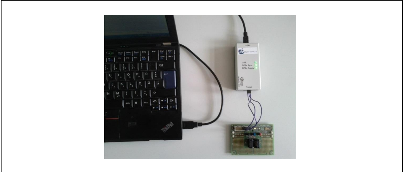
Figure 3 Interface Gen2 Box Connections to a PC and OTP Programming Board
