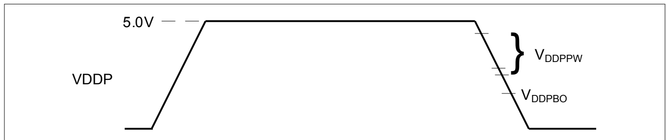
Figure 16 Supply Threshold Parameters
