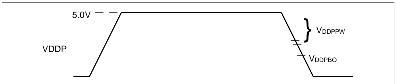
Figure 13 Supply Threshold Parameters
