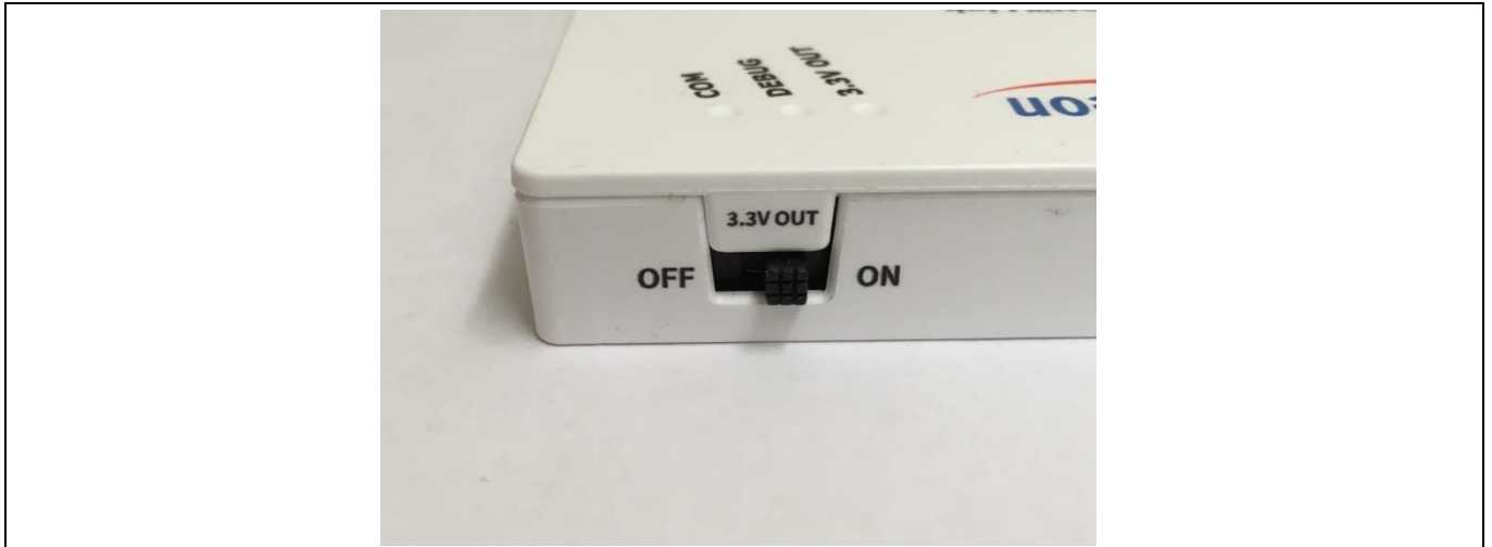
Figure 3 iMOTION™ Link “3.3V OUT” switch
