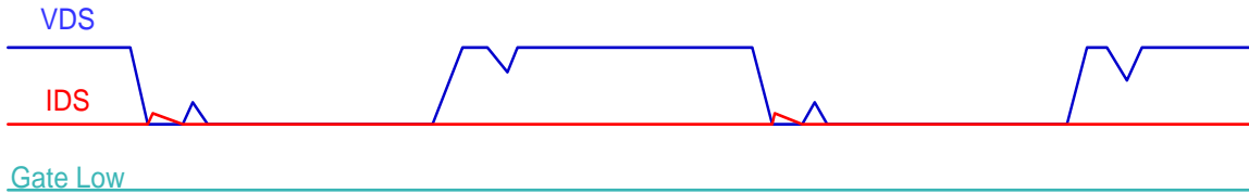
Figure 4: Waveform under MOT protection mode
