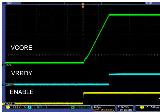
Figure 11: Enable-based Startup
