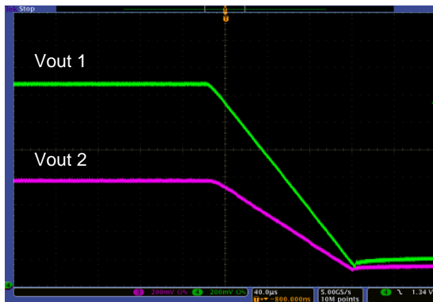
Figure 15: MPoL Tracking Shutdown
