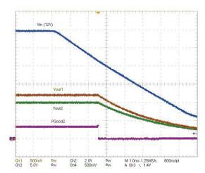
Figure 15: Vin based shutdown, the high side and low side FETs are turned off as soon as Vin falls below UVIO threshold.
