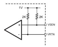
Figure 19: Output Voltage sensing impedance
