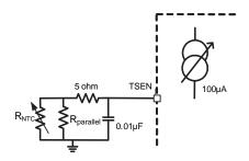
Figure 36: Temperature Sense NTC Network
