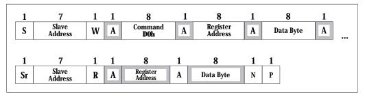
Figure 46: SMBus Process Call to Write an IR Register
