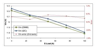
Figure 39: I2C Input Voltage Measurements
