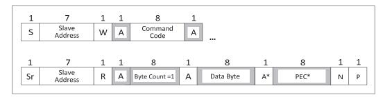
Figure 45: SMBus Block Read with Byte Count=1
