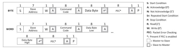
Figure 42: SMBus Write Byte/Word
