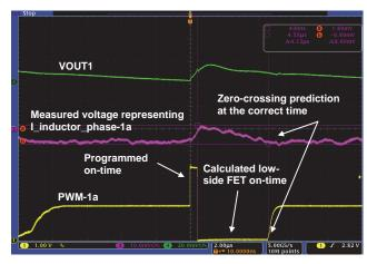
Figure 32: PS2 Active Diode Emulation Mode
