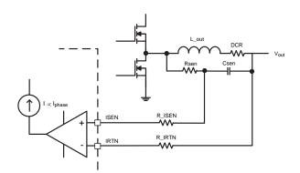
Figure 20: DCR Current Sensing
