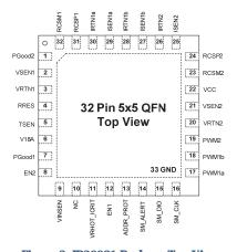
Figure 2: IR36021 Package Top View
