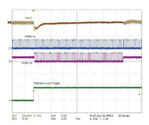
Figure 29: loop1 going from 1Φ to 2Φ operation due to a heavy load transient which causes Vout drop, 1Φ operation is resumed with a delay after Vout1 recoveres.
