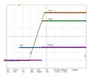
Figure 13: Enable-based startup, both loops start with a delay of 2.5ms from EN1 going high.
