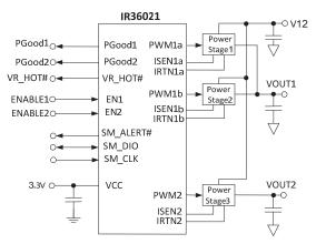
Figure 1: IR36021 Basic Application Circuit
