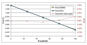
Figure 40: I2C Output Voltage Measurements
