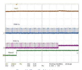
Figure 28: Phase Shed 2Φà 1Φ at startup
