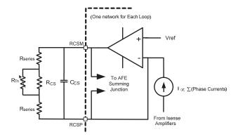
Figure 24: Load Line & Thermal Compensation
