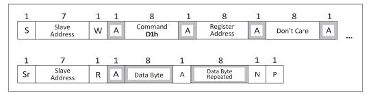
Figure 47: SMBus Process Call to Read an IR Register
