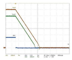
Figure 14: Enable based shutdown, both loops configured to follow EN1. Vout1 and Vout2 are ramped down to OV.
