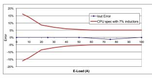
Figure 38: I2C I<sub>OUT</sub> Error using 10% DCR inductors
