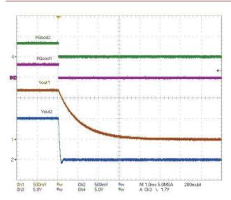
Figure 35: OCP on Loop #2 shuts down both loops
