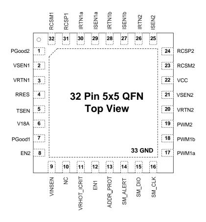
Figure 3: IR36021 Package Bottom View 5mm X 5mm QFN
