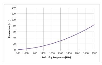
**Figure 17: Switching Frequency Resolution**
