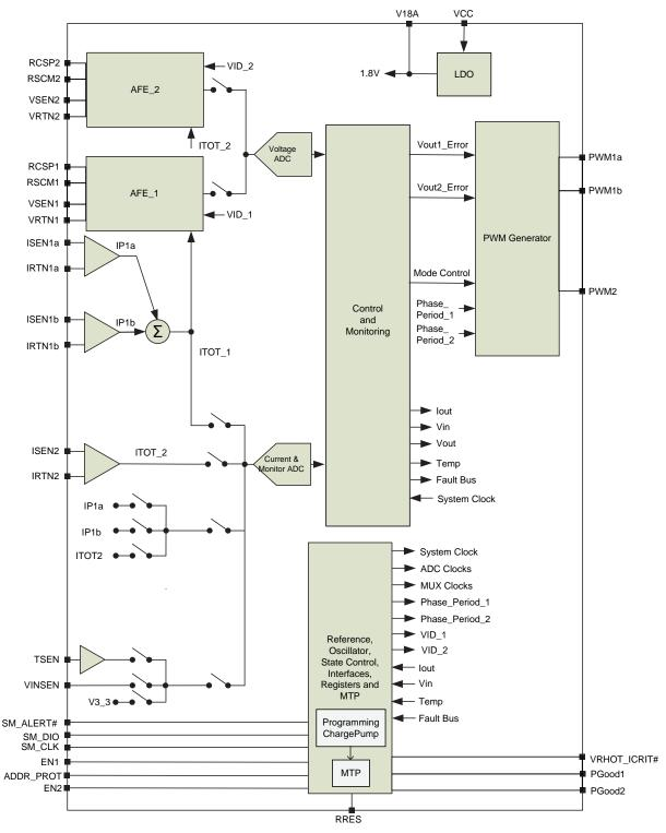
Figure 4: IR36021 Simplified Block Diagram
