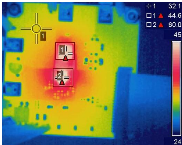
Figure 18: Thermal Image at V_{IN} = 12V , I_{OUT} = 6A (IR3863: 60^\circ C , Inductor: 45^\circ C , PCB: 32^\circ C )
