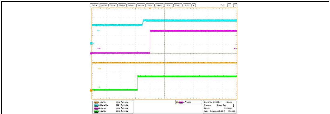
Figure 16 Pre-bias Start up at 0 A Load, (Ch1: PV in , Ch2: V out , Ch3:P Good ,Ch4:Enable)
