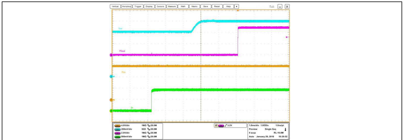
Figure 17 Pre-bias Start up at 0 A Load, (Ch1: PVin, Ch2: Vo, Ch3: PGood, Ch4: En)
