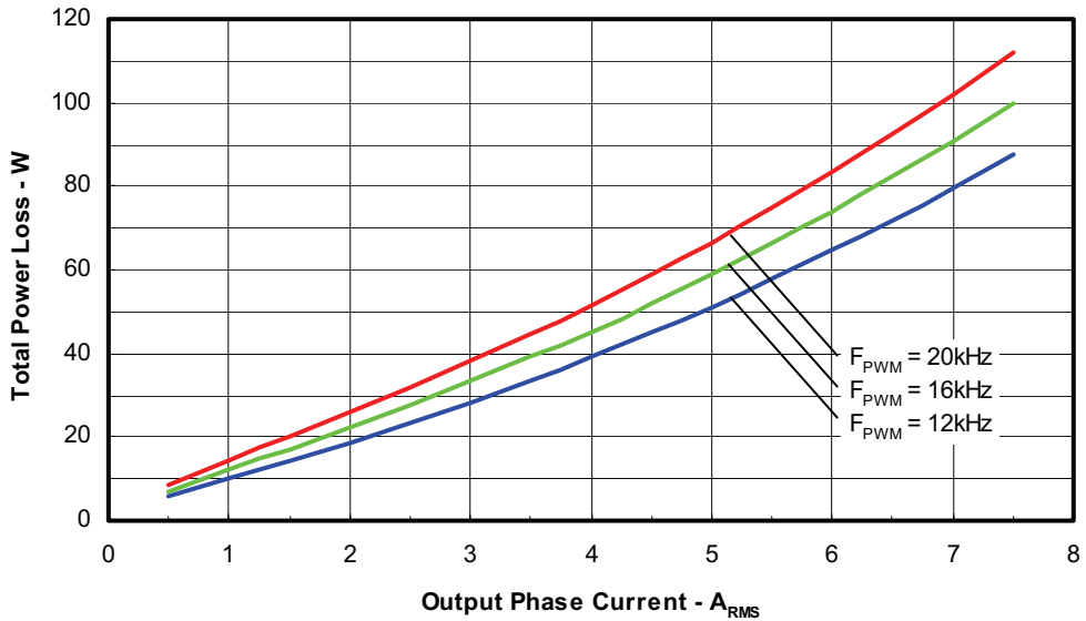
Figure 7. Total Power Losses vs. Output Phase Current Sinusoidal Modulation, V^+ = 400V , T_J = 150^\circ C , MI = 0.8 , PF = 0.6 , f_{mod} = 50Hz
