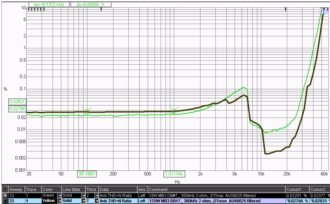
Figure 4 THD+N vs. Frequency at 10W and 125W
