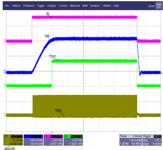
Ch1-Phase Voltage (10V/Div) Ch2-Vout(500mV/Div) Ch3-EN(2V/Div) Ch4-PGood(2V/Div)
