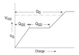
Fig 13a. Basic Gate Charge Waveform
