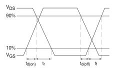
Fig 10b. Switching Time Waveforms
