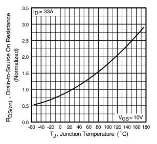
Fig 4. Normalized On-Resistance Vs. Temperature
