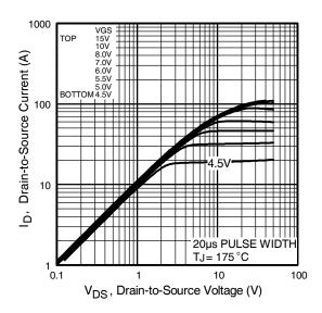
Fig 2. Typical Output Characteristics
