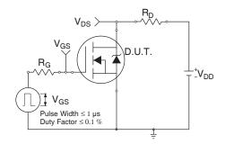
Fig 10a. Switching Time Test Circuit
