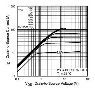
Fig 1. Typical Output Characteristics
