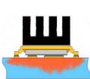
⑨ Mounted to a PCB with small clip heatsink (still air)
