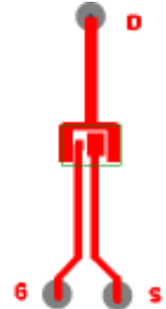
⑩ Mounted on minimum footprint full size board with metalized back and with small clip heatsink (still air)
