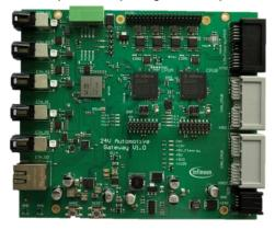
family, while supporting the latest communications interfaces, featuring a Gigabit Ethernet interface, multiple ISO 11898-1-compliant CAN FD channels, as well as LIN and Flexray channels. An additional eMMC interface for external flash interfacing enables local data storage, supporting software-over-theair update concepts. Realtek's RTL9047AA automotive Ethernet switch controller features five integrated
