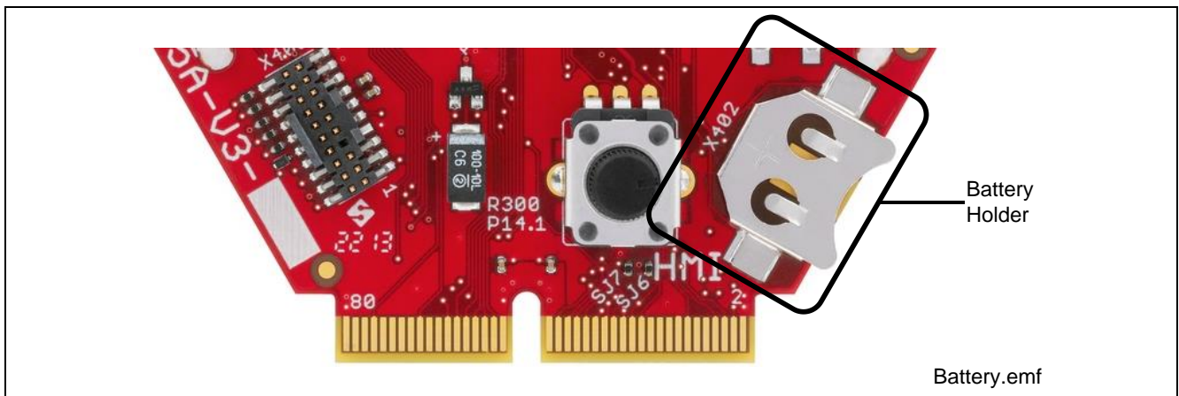
Figure 5 Battery (VBAT Supply)
