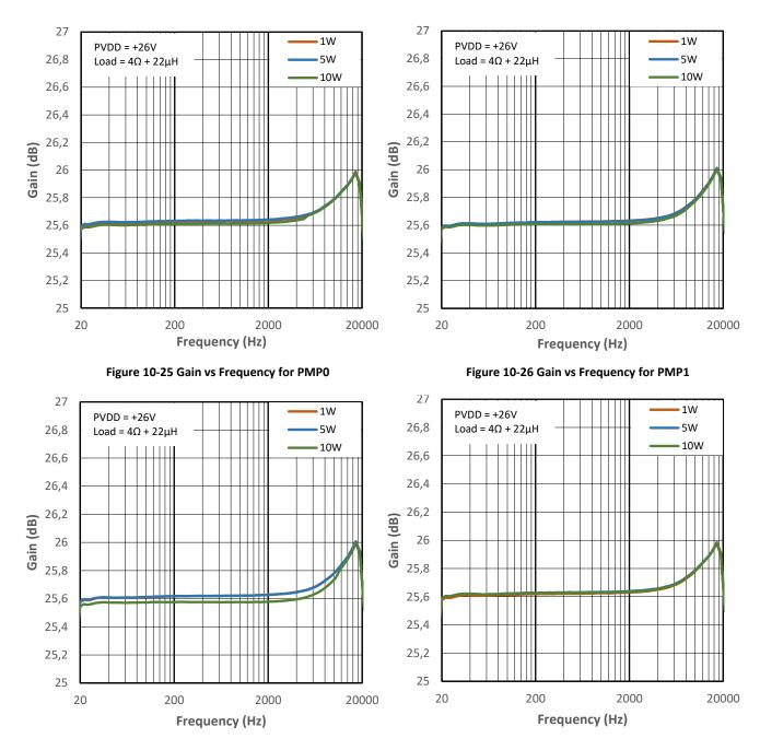
Figure 10-27 Gain vs Frequency for PMP2
