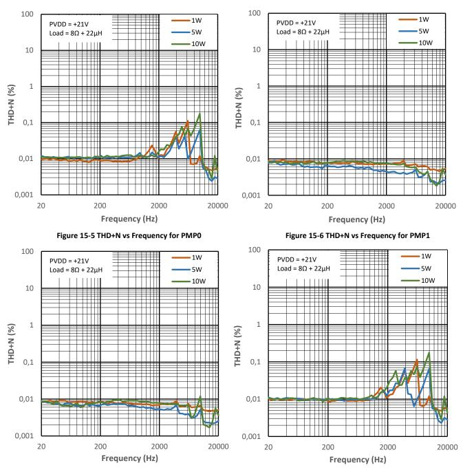
Figure 15-7 THD+N vs Frequency for PMP2
