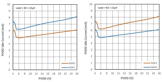
Figure 10-19 PVDD Idle Current vs PVDD for PMP0 & PMP1
