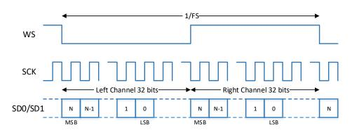
Figure 8-2 Timing diagram of left justified mode (default).
