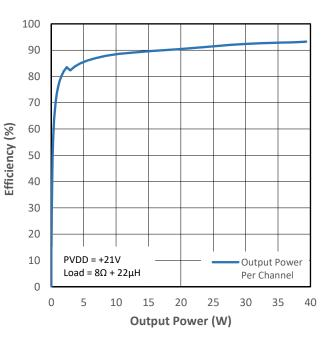
Figure 15-11 PMP2 Efficiency (VDD+PVDD) vs Output Power
