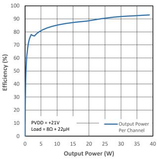
Figure 15-9 PMP0 Efficiency (VDD+PVDD) vs Output Power
