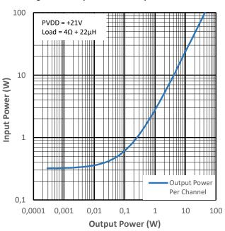
Figure 14-15 Input Power vs Output Power for PMP2
