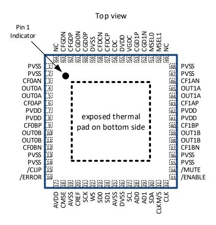
Figure 4-1 Pinout MA12070P
