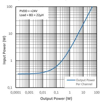
Figure 13-15 Input Power vs Output Power for PMP2
