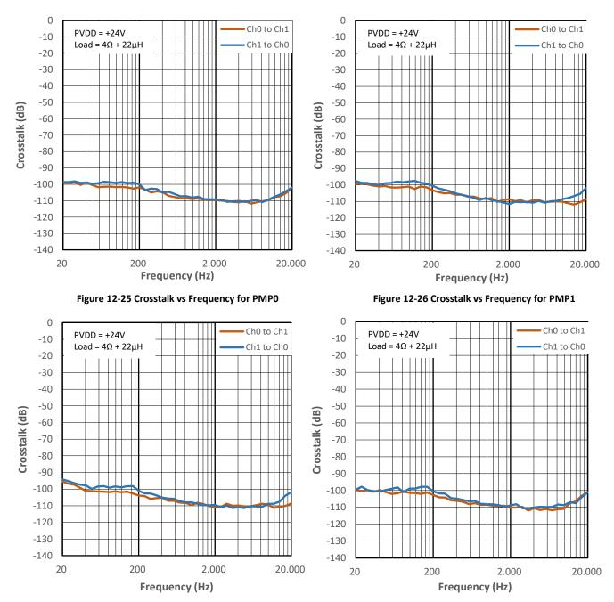
Figure 12-27 Crosstalk vs Frequency for PMP2
