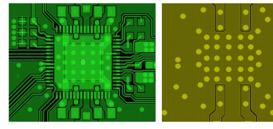
Figure 9-5 Example of 2-layer PCB layout, top and bottom layers
