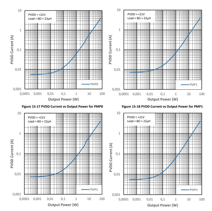
Figure 15-19 PVDD Current vs Output Power for PMP2
