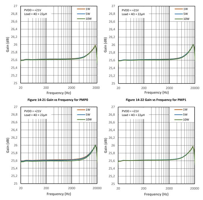
Figure 14-23 Gain vs Frequency for PMP2
