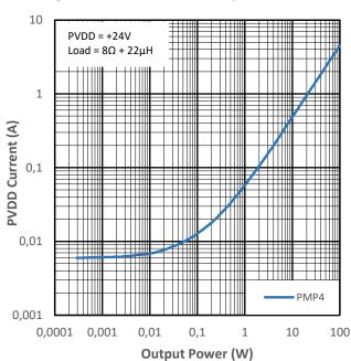
Figure 13-20 PVDD Current vs Output Power for PMP4
