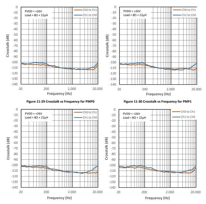
Figure 11-31 Crosstalk vs Frequency for PMP2
