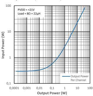
Figure 15-15 Input Power vs Output Power for PMP2
