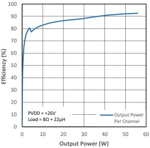
Figure 11-9 PMP0 Efficiency (VDD+PVDD) vs Output Power
