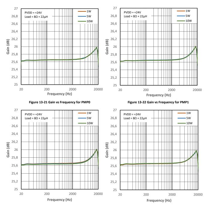
Figure 13-23 Gain vs Frequency for PMP2
