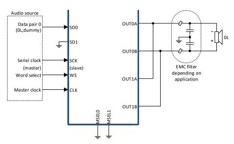
Figure 9-4 Parallel Bridge Tied Load (PBTL) configuration
