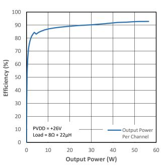
Figure 11-12 PMP4 Efficiency (VDD+PVDD) vs Output Power
