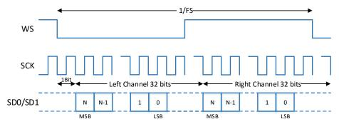
Figure 8-3 Timing diagram of I2S mode with 2x32 bit.
