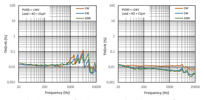
Figure 12-5 THD+N vs Frequency for PMP0
