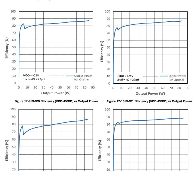
Figure 12-11 PMP2 Efficiency (VDD+PVDD) vs Output Power
