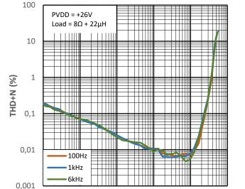
Figure 11-2 THD+N vs Output Power for PMP1
