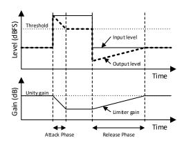
Figure 8-6 Example of limiter attack - and release behavior
