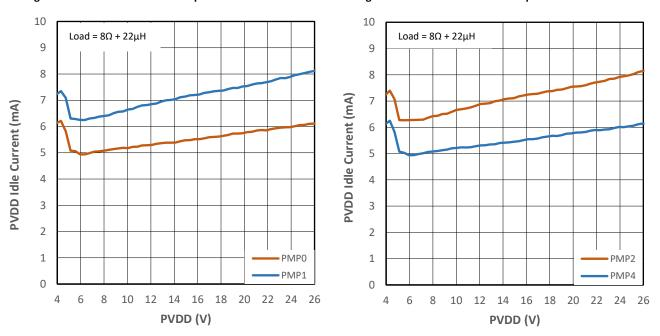
Figure 11-19 PVDD Idle Current vs PVDD for PMP0 & PMP1
