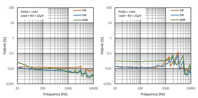
Figure 12-7 THD+N vs Frequency for PMP2
