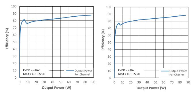
Figure 10-9 PMP0 Efficiency (VDD+PVDD) vs Output Power
