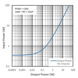
Figure 10-15 Input Power vs Output Power for PMP2
