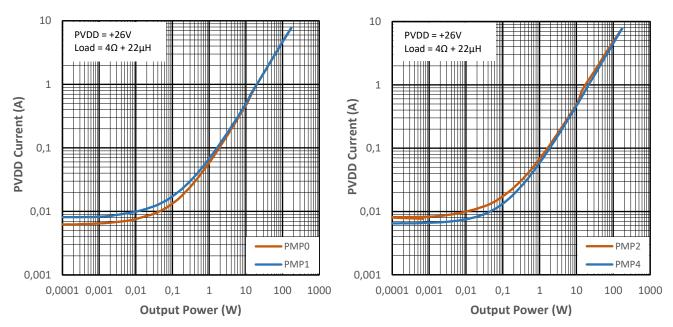
Figure 10-17 PVDD Current vs Output Power for PMP0 & PMP1 Figure 10-18 PVDD Current vs Output Power for PMP2 & PMP4
