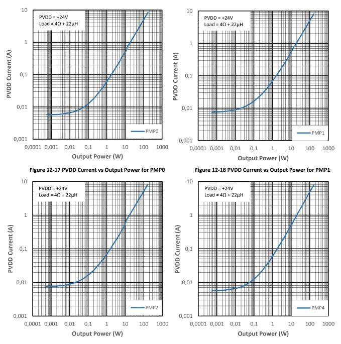
Figure 12-19 PVDD Current vs Output Power for PMP2
