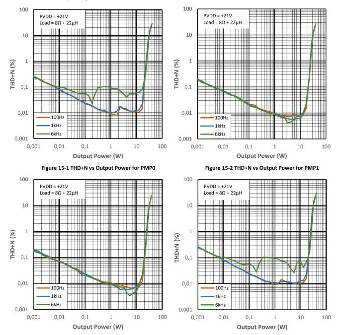
Figure 15-3 THD+N vs Output Power for PMP2
