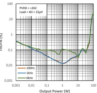
Figure 10-3 THD+N vs Output Power for PMP2
