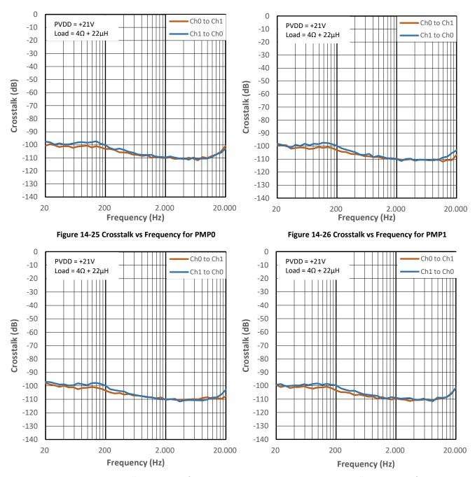
Figure 14-27 Crosstalk vs Frequency for PMP2
