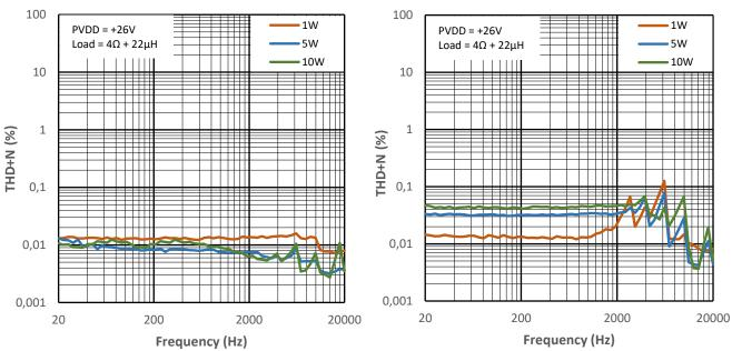
Figure 10-7 THD+N vs Frequency for PMP2
