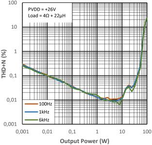
Figure 10-1 THD+N vs Output Power for PMP0
