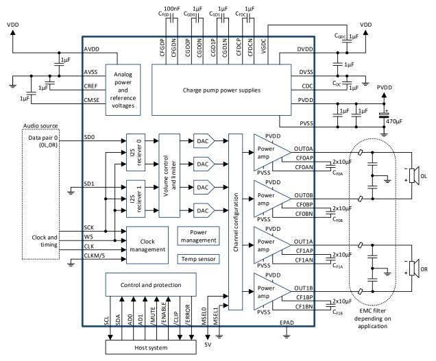
Figure 3-1 Typical application block diagram
