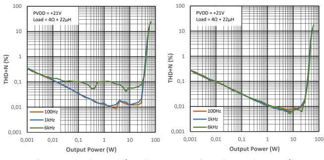
Figure 14-1 THD+N vs Output Power for PMP0
