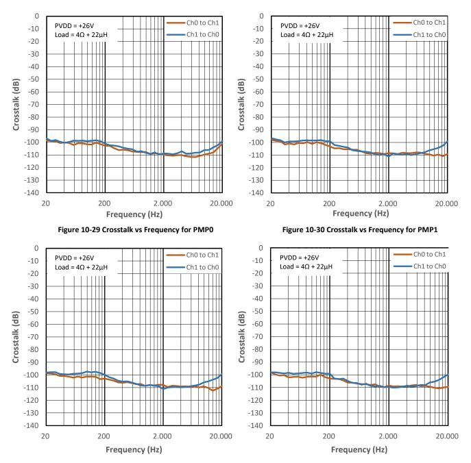
Figure 10-31 Crosstalk vs Frequency for PMP2
