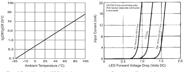
Figure 5. Typical Normalized Off-State Leakage
