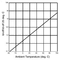
Figure 5. Typical Normalized Off-State Leakage
