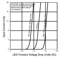
Figure 6. Input Characteristics (Current Controlled)
