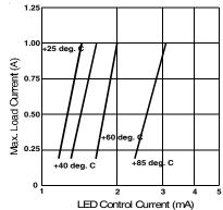
Figure 2. Typical Control Current Requirements
