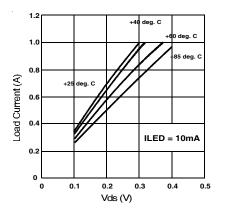
Figure 3. Typical On-Characteristics
