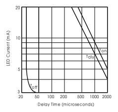
Figure 7. Typical Delay Times
