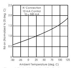
Figure 4. Typical Normalized On-Resistance
