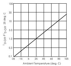
Figure 5. Typical Normalized Off-State Leakage
