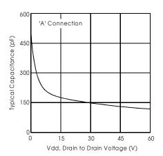
Figure 2. Typical Output Capacitance
