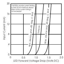
Figure 6. Input Characteristics (Current Controlled)
