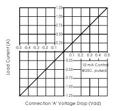
Figure 3. Linearity Characteristics
