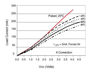
Figure 3. Typical On-Characteristic A Connection
