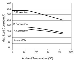
Figure 1. Current Derating Curve
