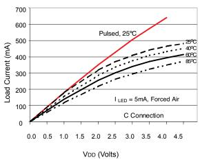
Figure 4. Typical On-Characteristic C Connection
