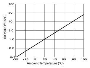
Figure 5. Typical Normalized Off-State Leakage
