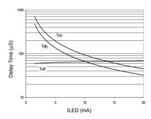
Figure 7. Typical Delay Times
