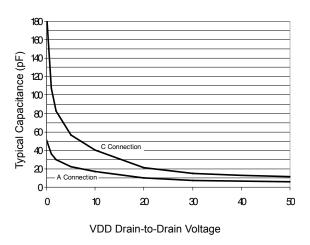
Figure 9. Typical Output Capacitance
