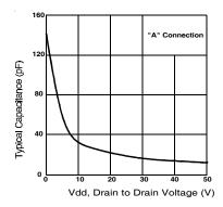
Figure 9. Typical Output Capacitance
