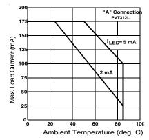
Figure 2. Typical Current Derating Curves
