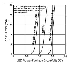
Figure 6. Input Characteristics (Current Controlled)
