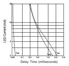
Figure 7. Typical Delay Times
