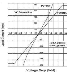
Figure 3. Linearity Characteristics
