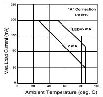
Figure 1. Typical Current Derating Curves
