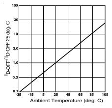
Figure 5. Typical Normalized Off-State Leakage
