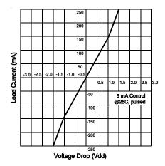
Figure 2. Linearity Characteristics
