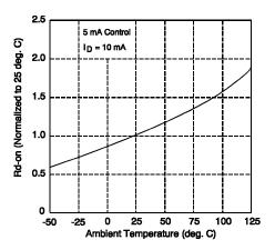
Figure 3. Typical Normalized On-Resistance
