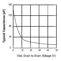
Figure 8. Typical Output Capacitance
