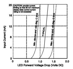
Figure 5. Input Characteristics (Current Controlled)
