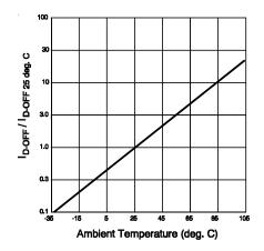
Figure 4. Typical Normalized Off-State Leakage
