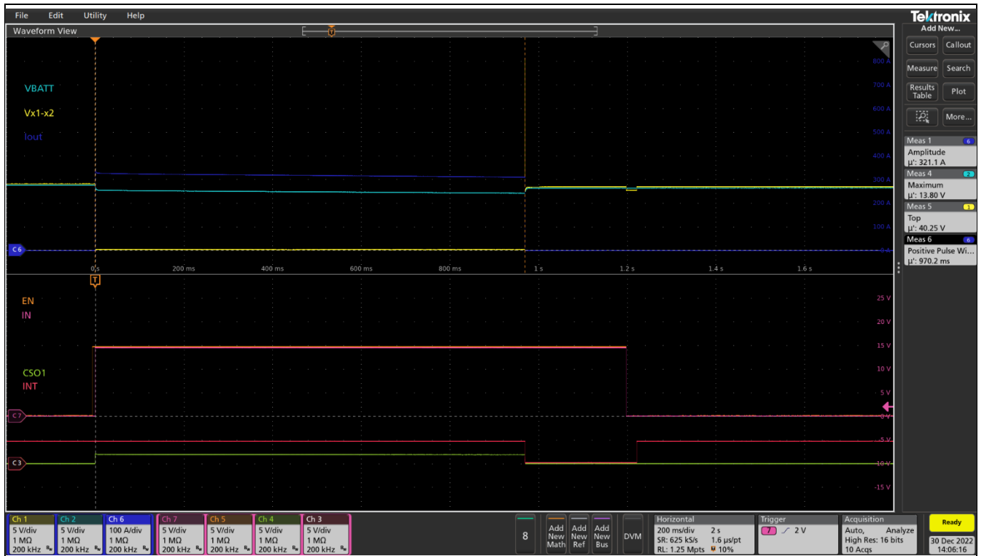
Figure 42 I-t wire protection test with circa 320 A scope depicting 200 ms/DIV
