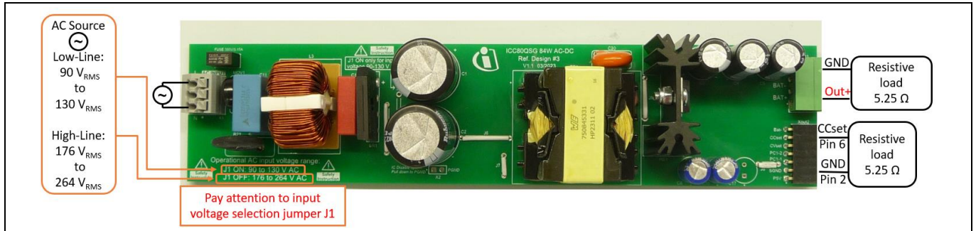
Figure 3 EMI test setup with full output power
