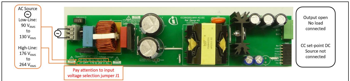
Figure 4 No-load system standby power test setup
