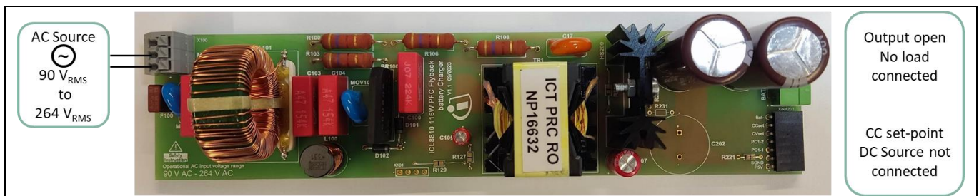
Figure 4 No-load system standby power test setup
