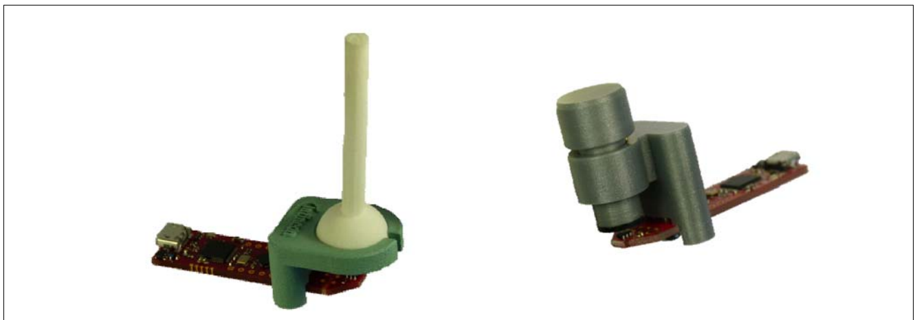
Figure 2 Magnet heads for the 3D Magnetic sensor 2 Go EvalBoard
