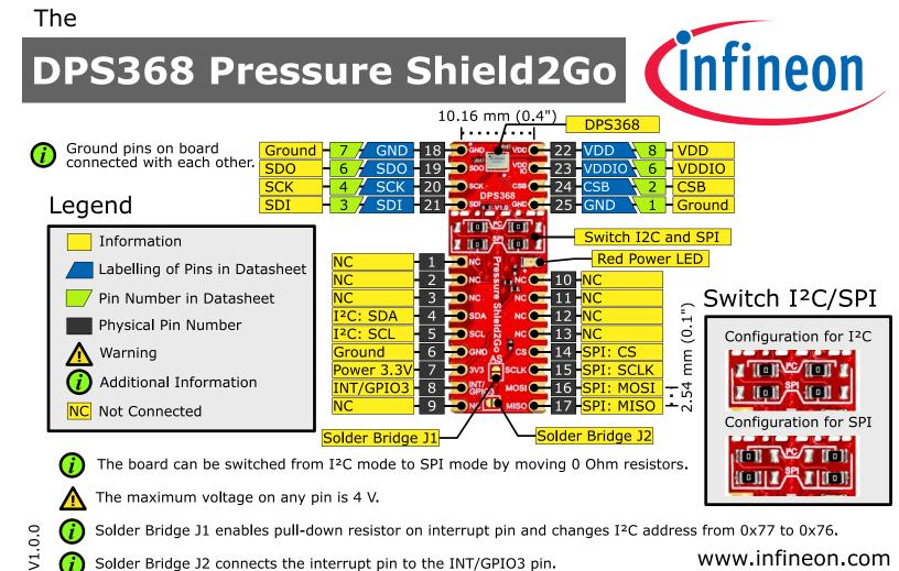
Solder Bridge J2 connects the interrupt pin to the INT/GPIO3 pin.
