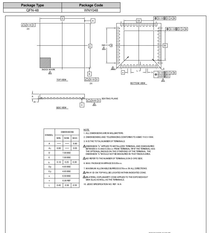
PACKAGE OUTLINE, 48 LEAD QFN 7.00X7.00X0.80 M M WNY048 4.65 X4.65 M M EPAD (SAWN) REV\*
