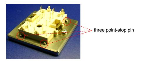
Note: If mechanical stops are used it is to be made certain that the ceramic edge of the module is not damaged.
