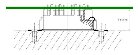
Bending and warping of the circuit board has to be avoided.
