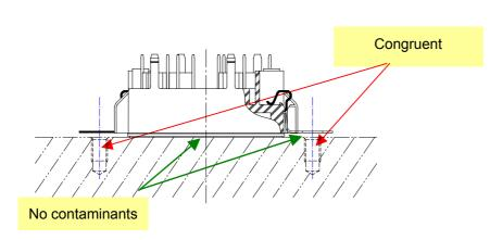
In order to position the module on the heat sink correctly a three pointstop pin on the heat sink is recommended.
