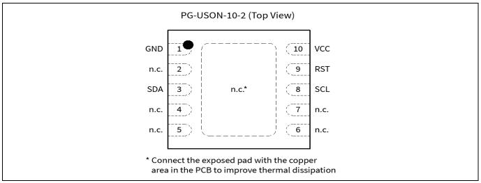
The following figure shows the PG-USON-10-2,-4 in top view:
