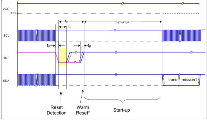
Figure 9 Startup of I2C Interface for Warm Resets
