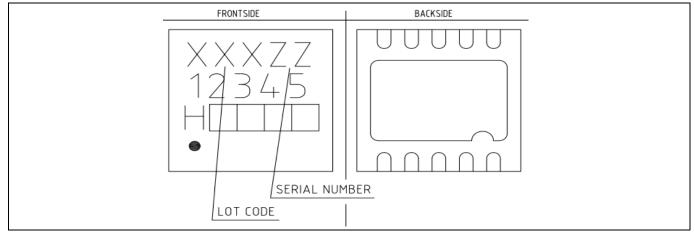
Figure 6 PG-USON-10-2,-4 sample marking pattern
