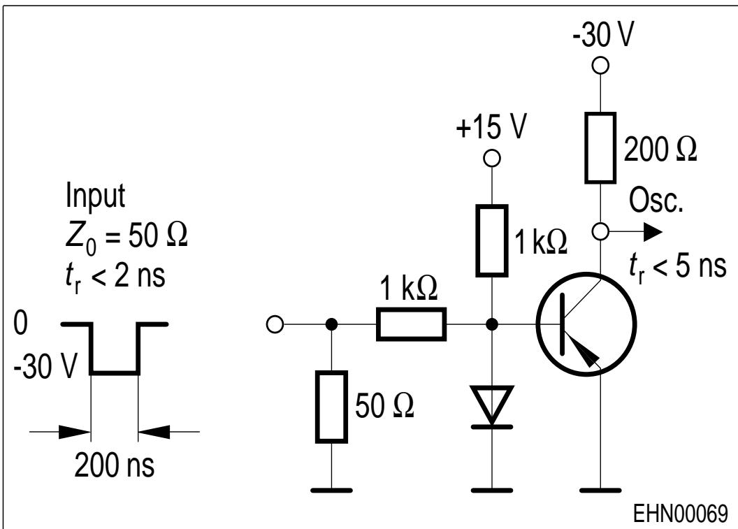
**Oscillograph:**  $R > 100$ ,  $C < 12\text{pF}$ ,  $t_r < 5\text{ns}$
