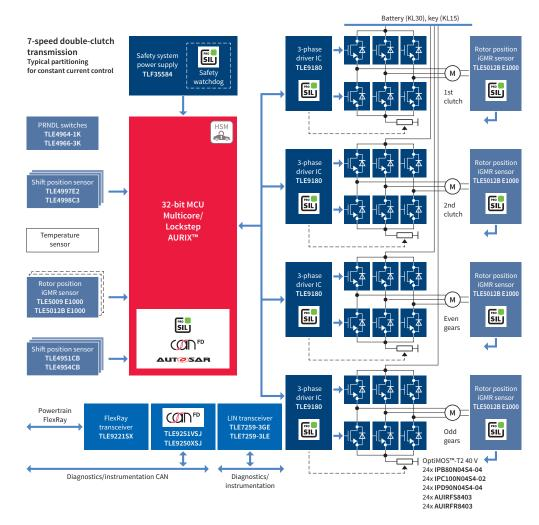
Thanks to its state-of-the-art safety features, the new TriCore<sup>™</sup> AURIX<sup>™</sup> family enables systems to achieve the highest safety level up to ASIL-D. The rich scalability of the AURIX<sup>™</sup> family permits a platform approach that meets the needs of a range of transmission systems. Furthermore, the hot temperature package and bare die solutions enable AURIX<sup>™</sup> to be used in both attached and integrated control units.
