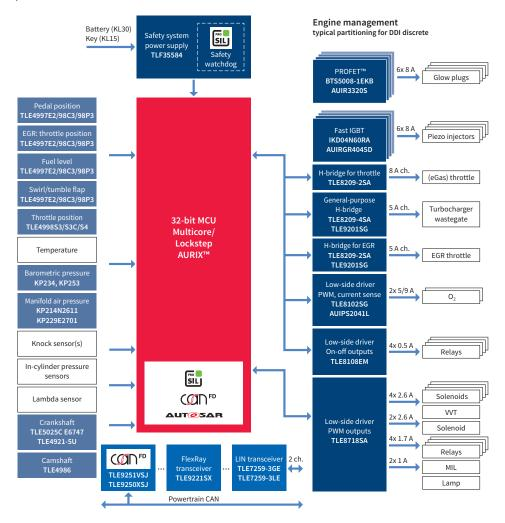
Thanks to its state-of-the-art safety features, the TriCore™ AURIX™ family enables systems to achieve the highest safety level up to ASIL-D. The scalable AURIX™ family includes the GTM, the de-facto industry standard timing module that supports highly complex engine management, while meeting the market's most stringent emissions regulations.
