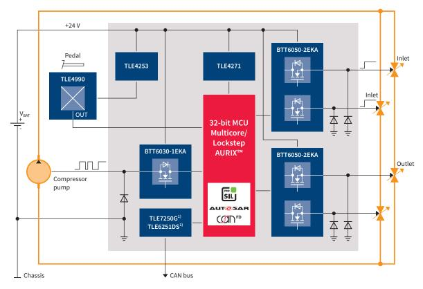
Pneumatic management system is typically chosen for its cost effectiveness and ease of integration (no need for a reservoir) compared to its hydraulic counterpart.
