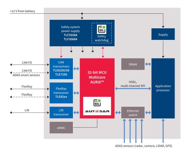
The new TriCore™ AURIX™ TC3xx family offers a scalable product portfolio to address the needs of sensor fusion applications, from stand-alone object fusion to companionship for a high-end AD ECU.
