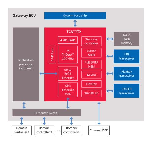
In gateway applications, AURIX™ TC3xx microcontrollers support the latest communications interfaces and feature a Gigabit Ethernet interface, up to 12 ISO 11898-1-compliant CAN FD channels and up to 24 LIN channels. An additional eMMC interface for external flash interfacing enables local data storage, supporting software-over-the-air update concepts.
