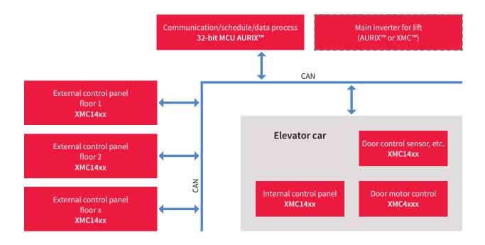
Modern elevators have strong safety requirements. The new TriCore<sup>™</sup> family AURIX<sup>™</sup> with state-of-the-art safety features enables your system to meet the highest safety levels that are required in your system.
