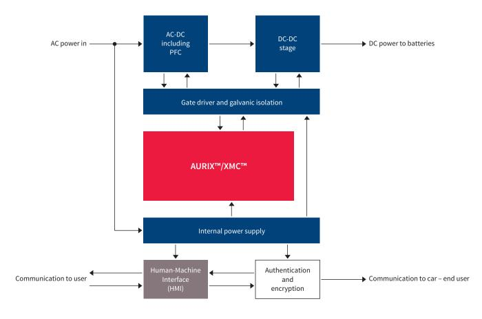
Off-board charging, where users can charge plug-in hybrids and pure EVs in private garages and open parking lots, demands an optimized solution with high MCU switching frequency to stay efficient and cost competitive. The Infineon XMC<sup>™</sup> family is the answer! If you have security or safety requirements, you can scale from XMC<sup>™</sup> family to AURIX<sup>™</sup> to support your solution.
