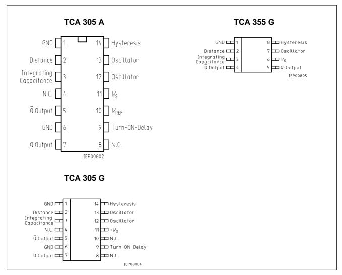
Pin Configurations (top view)
