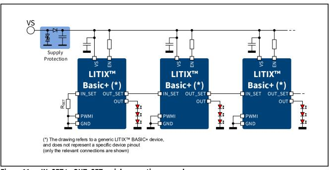
Figure 11 IN\_SET to OUT\_SET serial connection example
