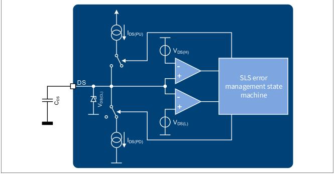
Figure 23 DS pin (block diagram)
