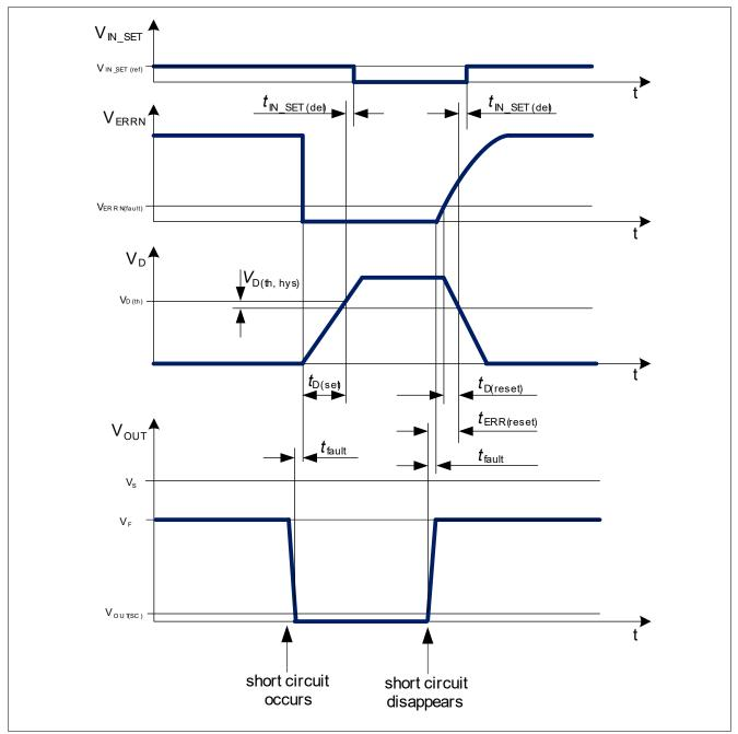
Figure 19 Short circuit to GND condition timing diagram example (D-pin not connected or connected to external capacitor to GND, V<sub>Fxvz</sub> represents the forward voltage of the output loads)
