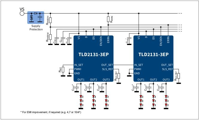
Figure 26 Application diagram example
