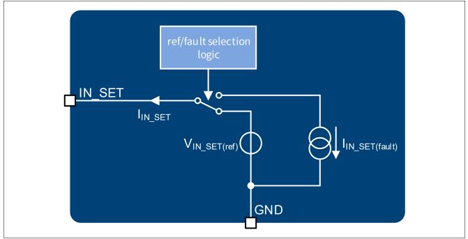
Figure 6 IN\_SET pin block diagram
