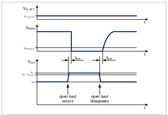
Figure 20 Open load condition timing diagram example (D-pin connected to GND, V<sub>F</sub> represents the forward voltage of the output load)
