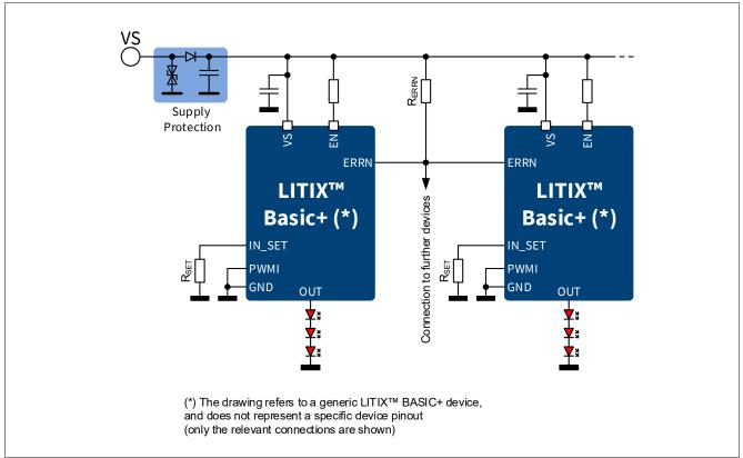
Figure 16 Shared error network principle between LITIX<sup>™</sup> Basic+ family devices
