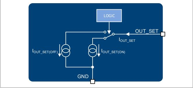
Figure 10 OUT\_SET pin block diagram
