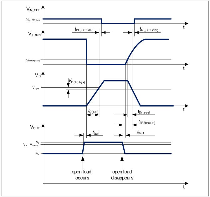
Figure 18 Open load condition timing diagram example (D-pin unconnected or connected to external capacitor to GND, V<sub>F</sub> represents the typical forward voltage of the output load)
