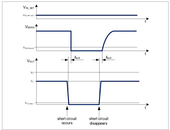
Figure 21 Short circuit condition timing diagram example (D-pin connected to GND, V<sub>F</sub> represents the forward voltage of the output load)
