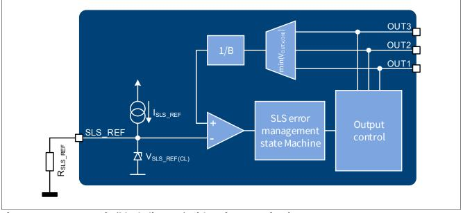
Figure 22 SLS\_REF pin (block diagram) with resistor termination
