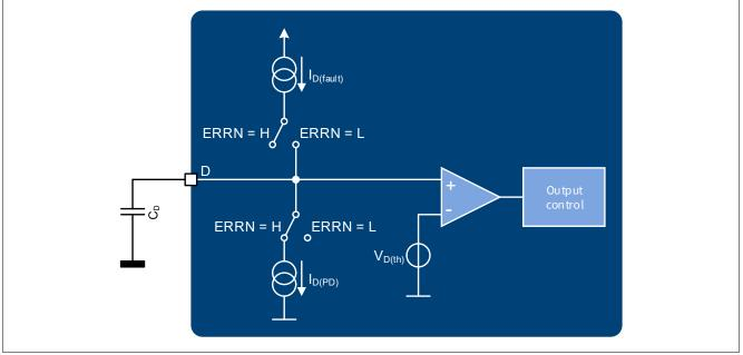
Figure 17 D-pin (block diagram).
