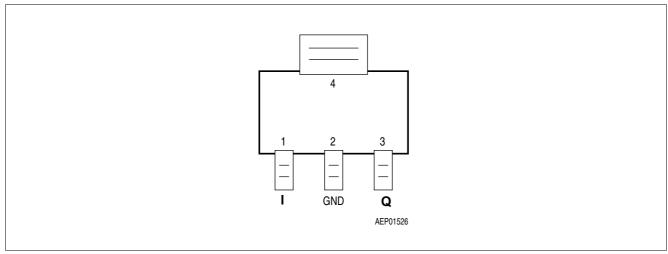
Figure 2 Pin Configuration
