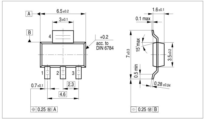
Figure 4 PG-SOT223-4 (Plastic Small Outline Transistor)
