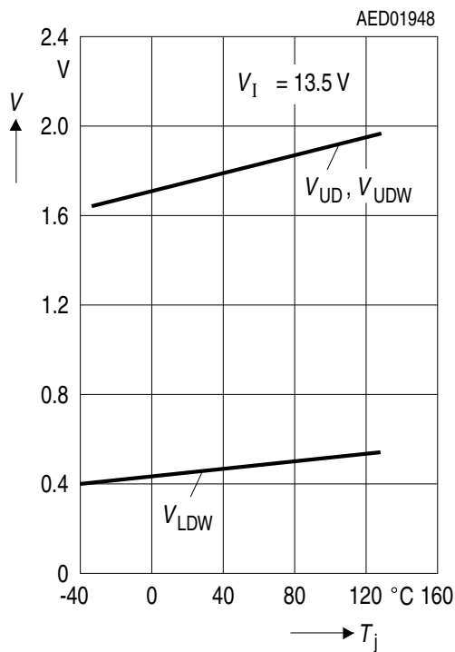
Switching voltage V_{UD} and V_{LDW} versus junction temperature T_j
