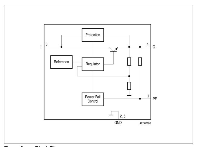
Figure 2 Block Diagram
