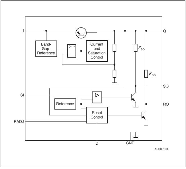
Figure 1 Block Diagram TLE 4299 G
