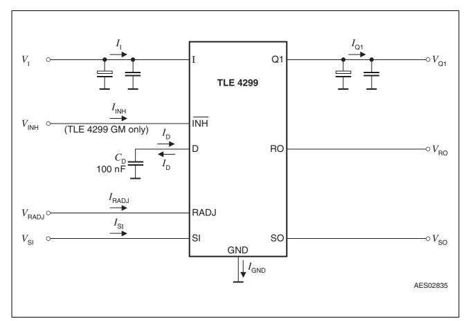
Figure 5 Measurement Circuit
