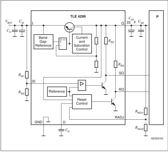
Figure 6 Application Diagram TLE 4299 G
