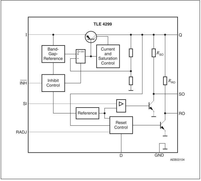
Figure 2 Block Diagram TLE 4299 GM
