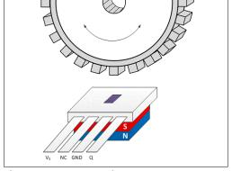
Figure 1-5 Wheel with sensor
