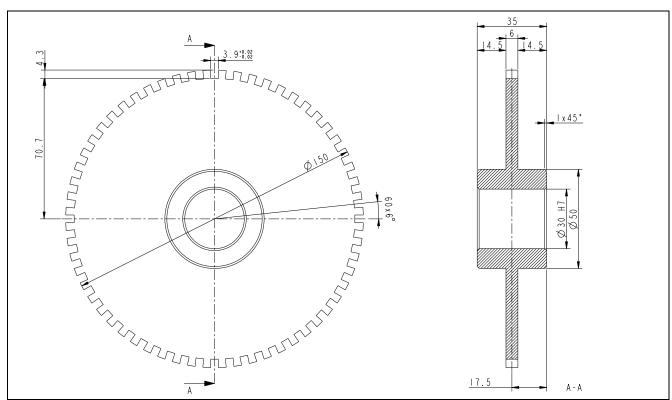
Figure 2-2 Infineon reference toothed wheel: dimension in mm
