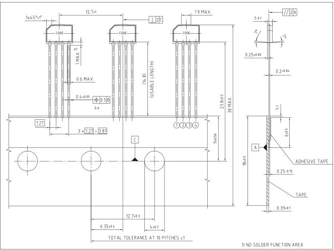
Figure 3-3 PG-SSO-4-1 packaging, dimensions in mm
