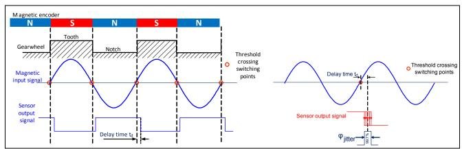
Figure 2-1 Phase error and delay time definition
