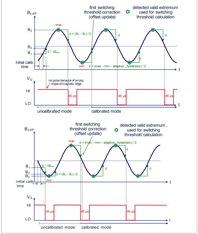
Figure 5 Operating Phases - Power-on to Running Phase
