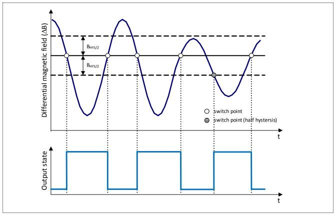
Figure 9 Hidden Hysteresis in protocol-variant without direction detection
