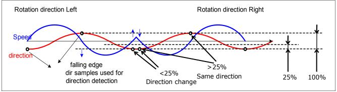
Figure 8 Direction Threshold Level
