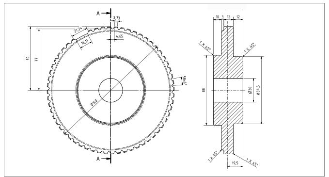
Figure 2 OEM-crankshaft wheel (outer diameter = 160mm)
