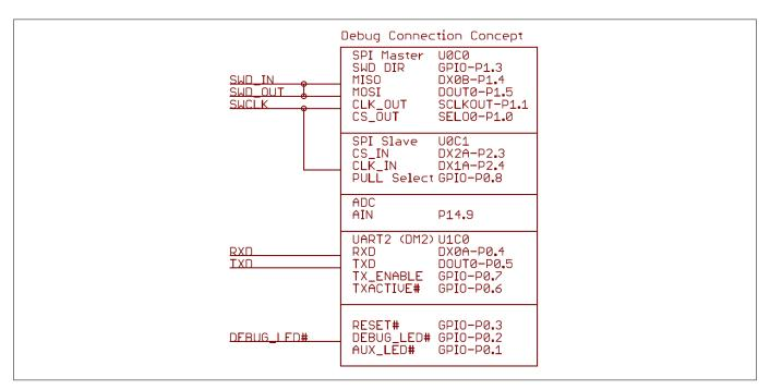
Figure 13 Sketch of the debug connection
