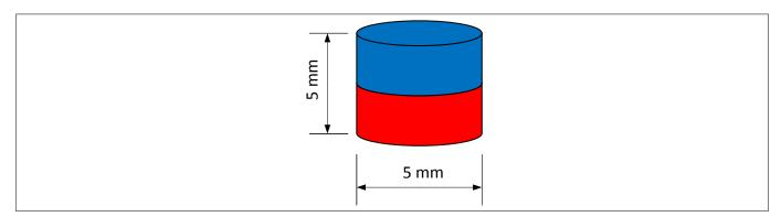
Figure 6 Magnet used in the linear slider extension
