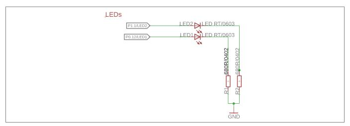
Figure 11 EvalBoard schematic: the LEDs for user configuration (connected to XMC1100 pins)
