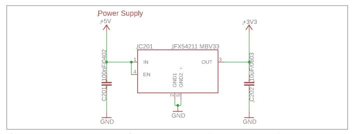
Figure 10 EvalBoard schematic: the voltage regulator (for the power supply)
