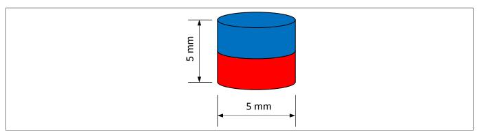
Figure 3 Magnet used in the Joystick extension
