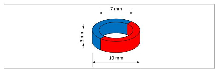
Figure 5 Magnet used in the out of shaft extension
