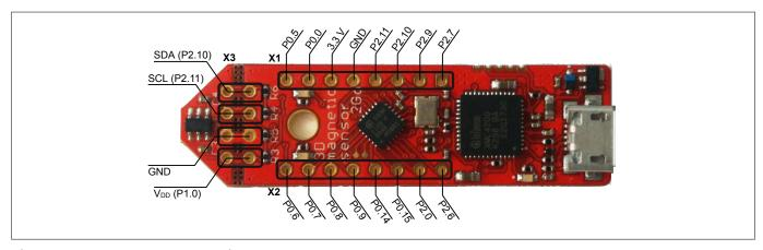
Figure 8 EvalBoard pin header connectors
