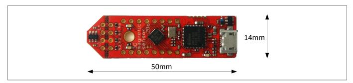
Figure 1 3D Magnetic Sensor 2 Go EvalBoard
