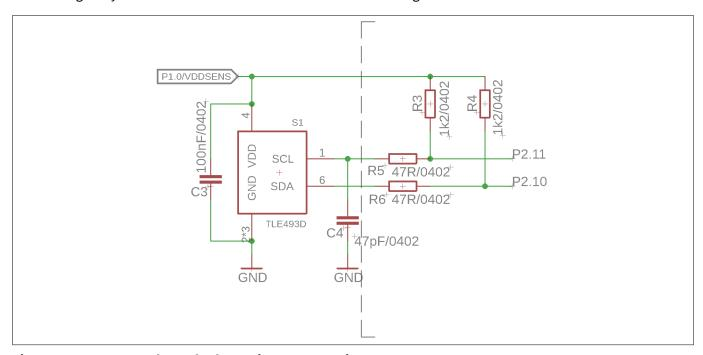
Figure 9 EvalBoard schematic: 3D magnetic sensor
