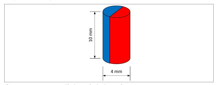
Figure 4 Magnet used in the rotation knob extension
