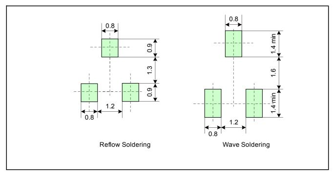
Figure 7 Footprint SC59 (SOT23 compatible)
