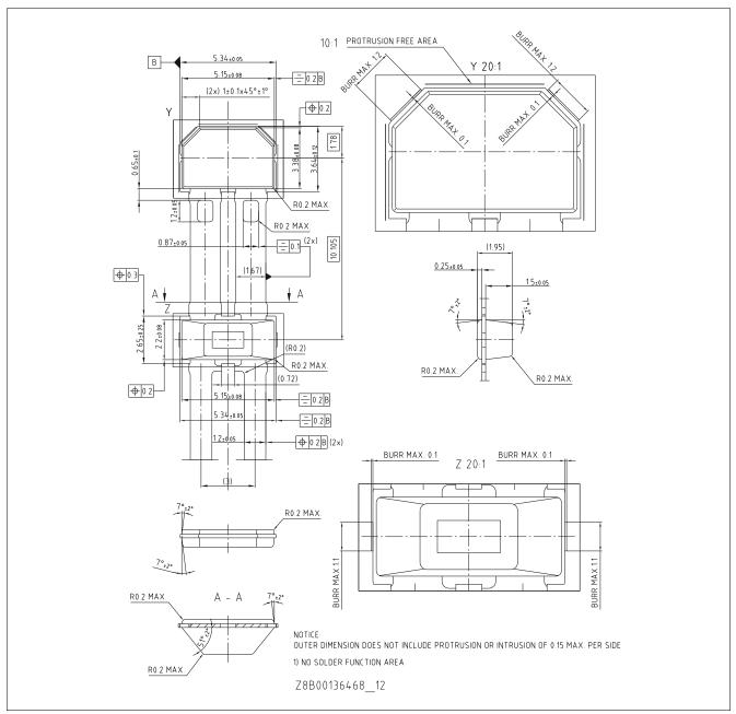
Figure 14 PG-SSO-2-53 package outline, dimensions in mm.
