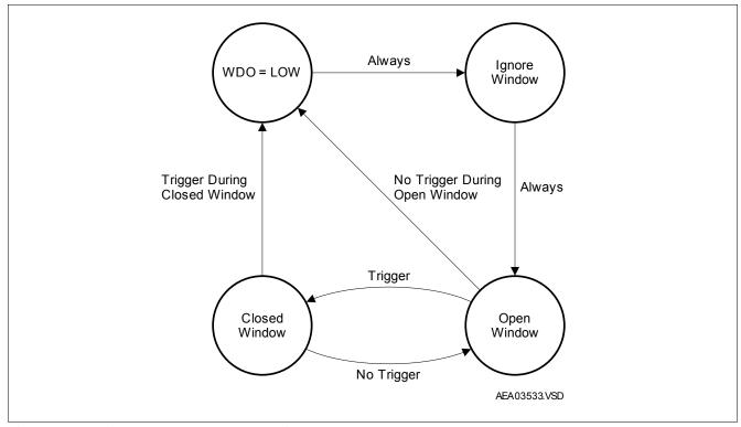
Figure 8 Window Watchdog State Diagram
