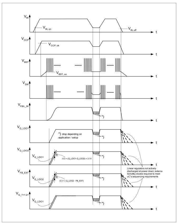
Figure 4 Power Sequencing of the TLE7368
