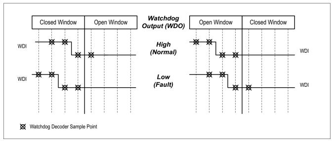
Figure 9 Window Watchdog Input Signal Validation
