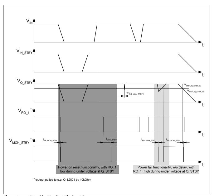
Figure 7 Stand by Monitor Timing Diagram
