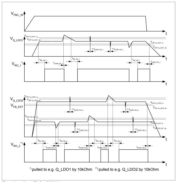
Figure 5 Reset Timing TLE7368
