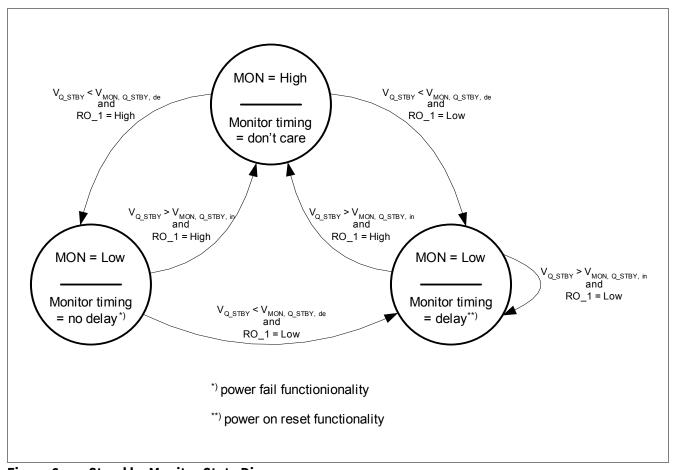
Figure 6 Stand by Monitor State Diagram
