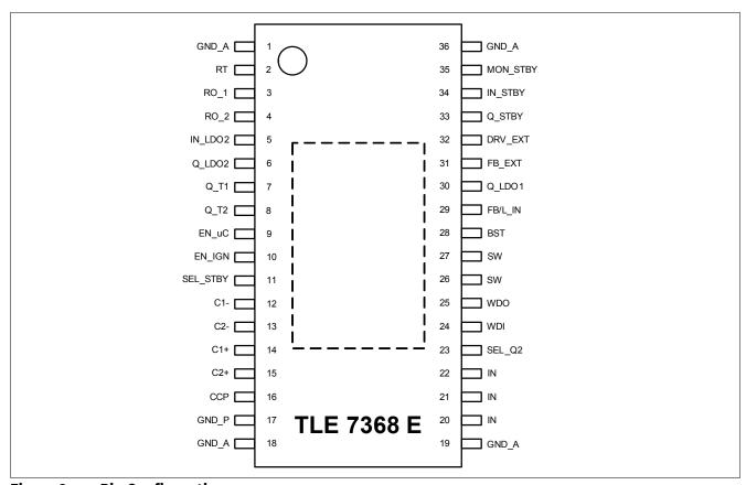
Figure 2 Pin Configuration
