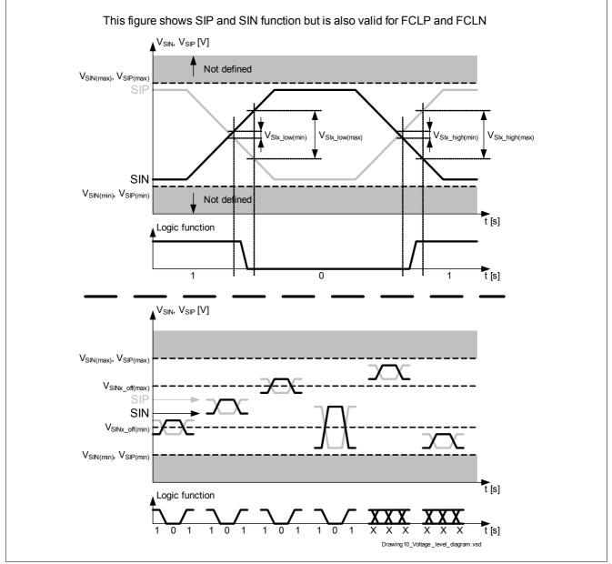
Figure 56 Voltage level diagram
