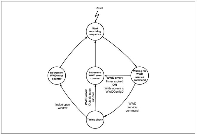
Figure 7 State Diagram of the Window Watchdog Module
