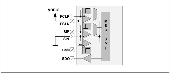
Figure 66 Block diagram of the SPI interface
