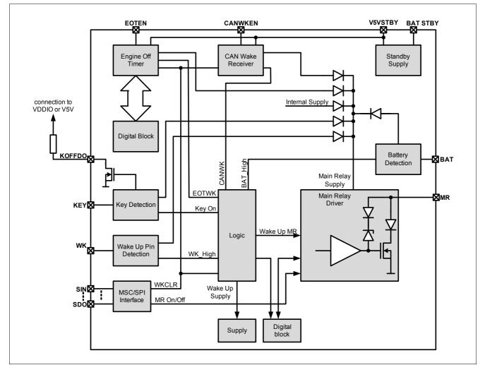
Figure 14 Block Diagram of the Key Detection, Wake-up Detection and Main Relay Driver
