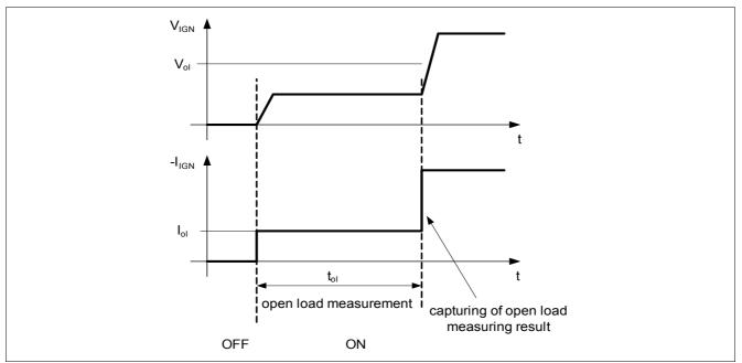
Figure 40 Ignition Output Open Load Detection
