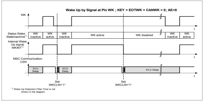
Figure 21 Functional Diagram for Internal Wake Signal
