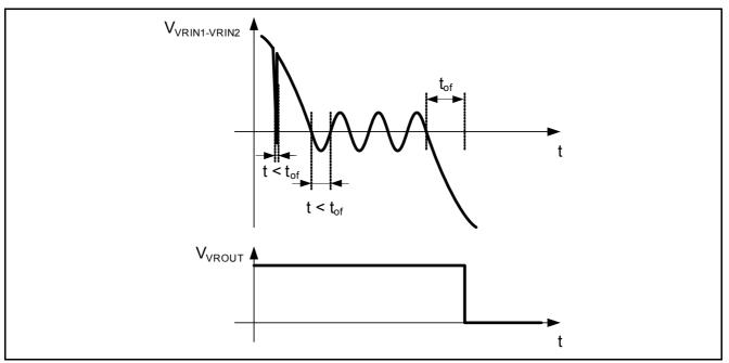
Figure 43 Output Filter Behavior
