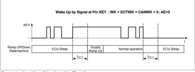
Figure 16 Function of Key detection filter time
