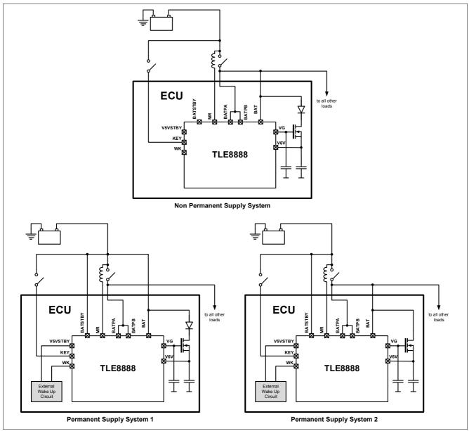
Figure 69 Application Diagram Supply Systems
