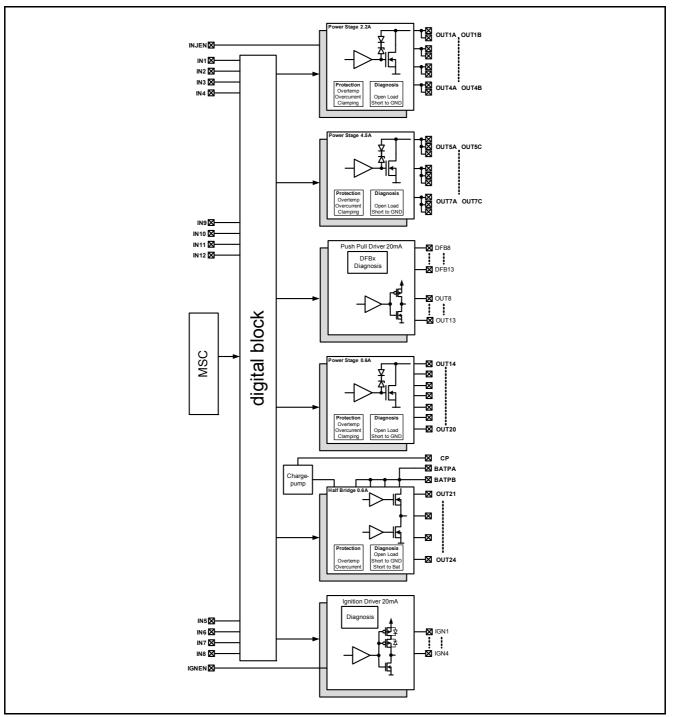
Figure 28 Block Diagram of the Power stages
