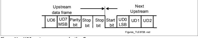
Figure 61 MSC upstream communication flow
