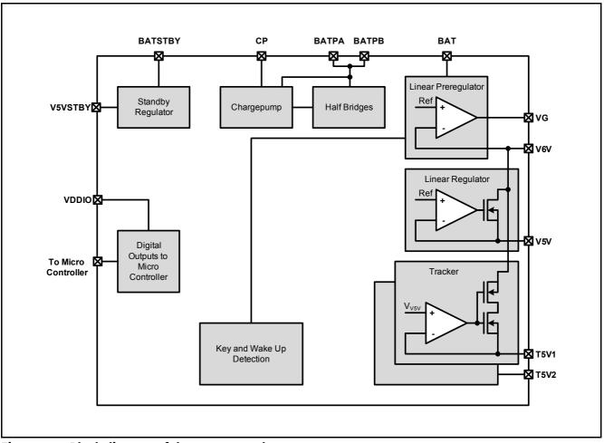
Figure 27 Block diagram of the power supply
