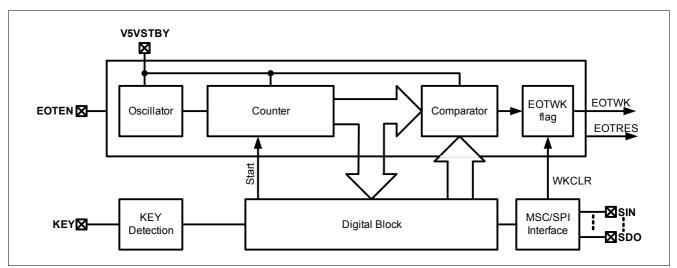
Figure 23 Block Diagram Engine Off Timer
