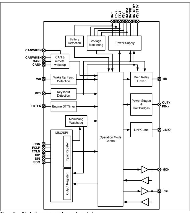
Figure 3 Block diagram operation mode control
