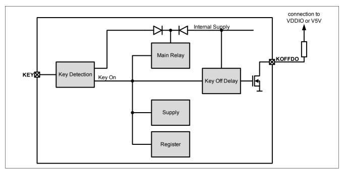
Figure 15 Block Diagram of the Key Detection
