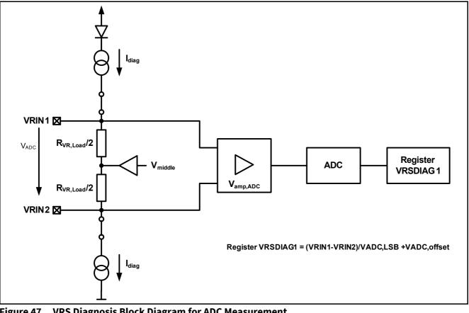
VRS Diagnosis Block Diagram for ADC Measurement Figure 47
