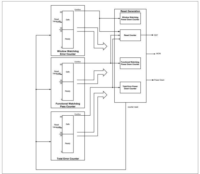
Figure 11 Block diagram of the Reset Generation
