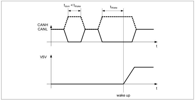
Figure 52 CAN Remote Wake-up
