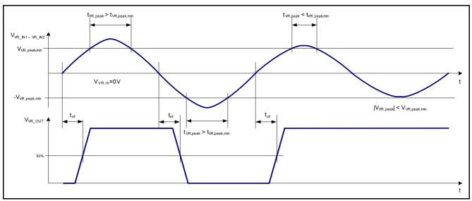
Figure 42 Timing Characteristics of the VR Sensor Interface
