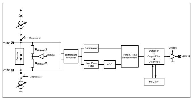
Figure 41 VR Sensor Interface Block diagram
