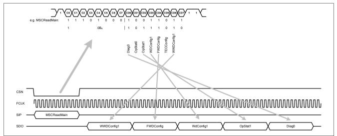
Figure 65 Example of a Multi read Command
