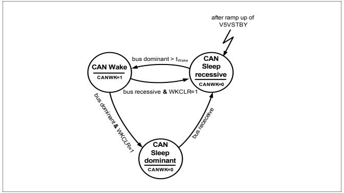
Figure 53 CAN Wake-up State machine
