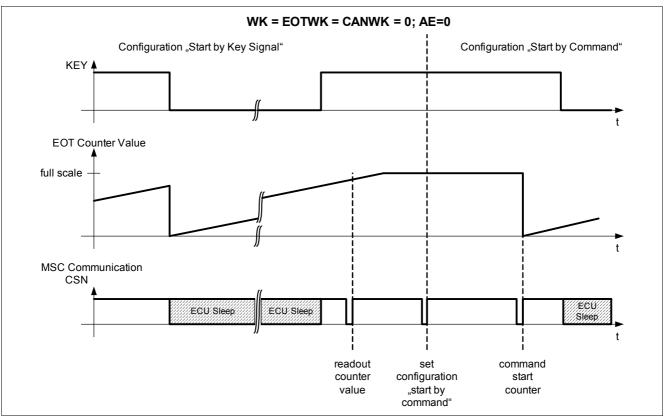
Figure 24 Function Diagram Engine Off Timer Counter Mode
