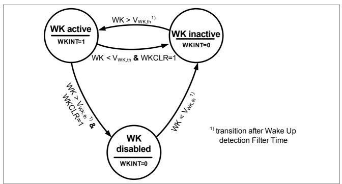
Figure 20 State Diagram of the Wake State Machine for Internal Wake Signal
