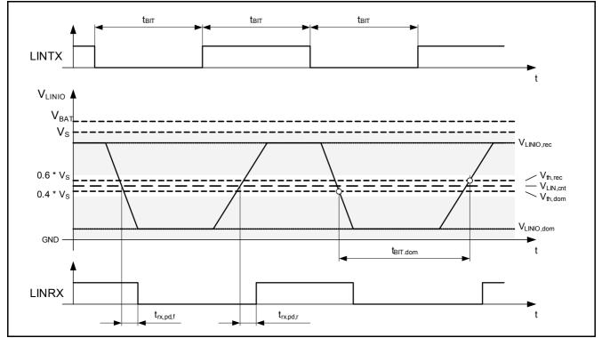
Figure 50 Timing Diagram of the LIN Interface
