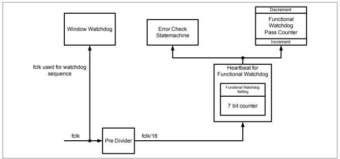
Figure 13 Clock Generation for the Watchdog Module
