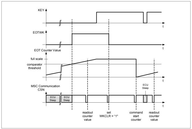
Figure 26 Function Diagram Engine Off Timer Comparator Mode
