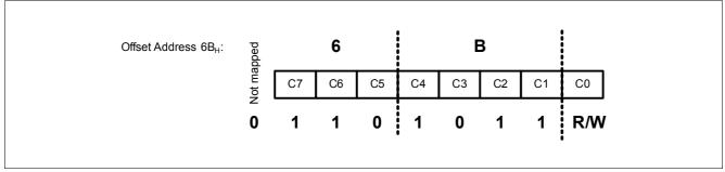
Figure 64 Mapping Offset Address to the Command Bits
