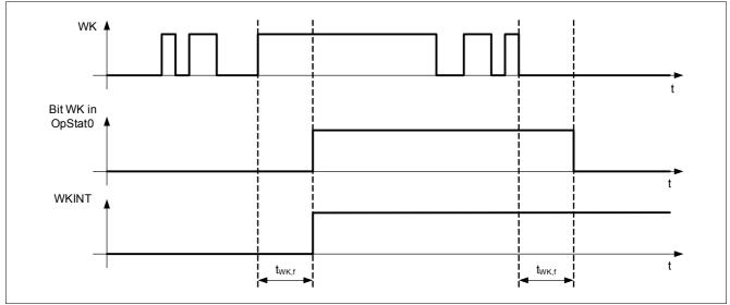
Figure 19 Function of WK detection filter time
