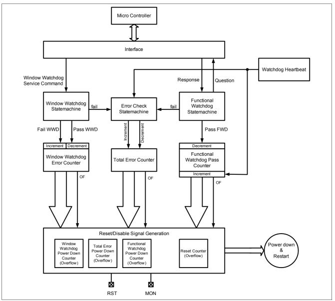
Figure 6 Block diagram of the Monitoring Watchdog Function
