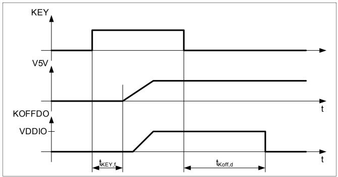
Figure 17 Timing Diagram of the Key Off Delay
