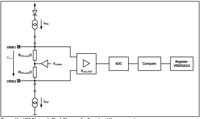
Figure 46 VRS Diagnosis Block Diagram for Open Load Measurement
