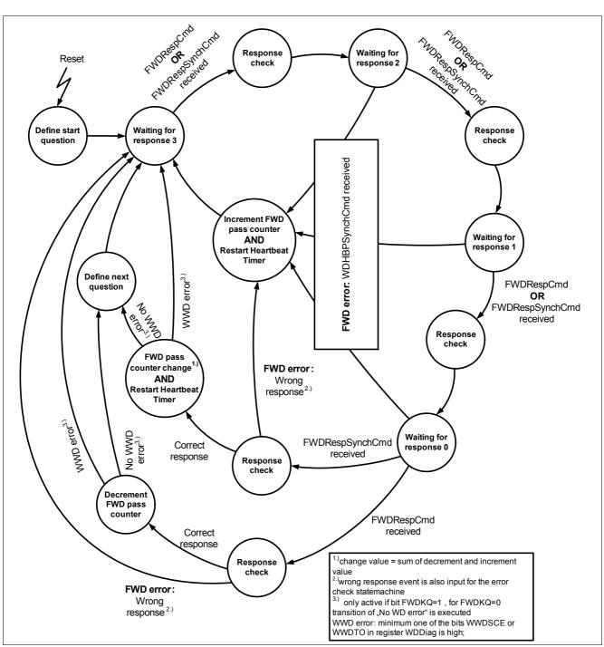
Figure 9 Functional Watchdog State diagram
