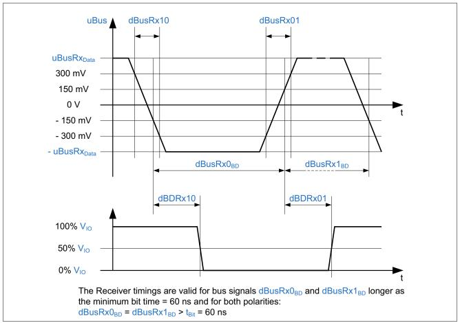
Figure 44 Receiver timing characteristics
