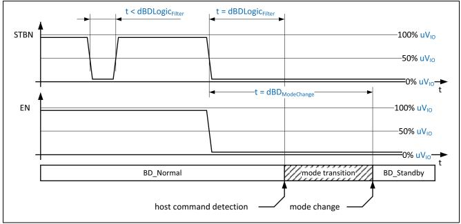
Figure 10 Example of a valid host command
