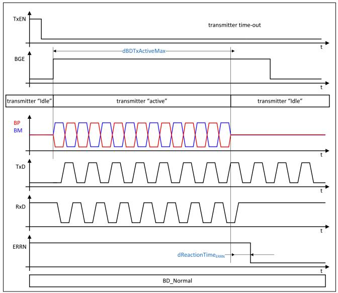
Figure 39 Transmitter time-out function
