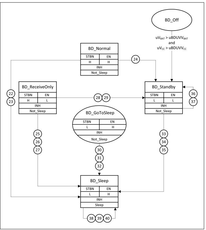
Figure 35 Operating mode changes by undervoltage flag
