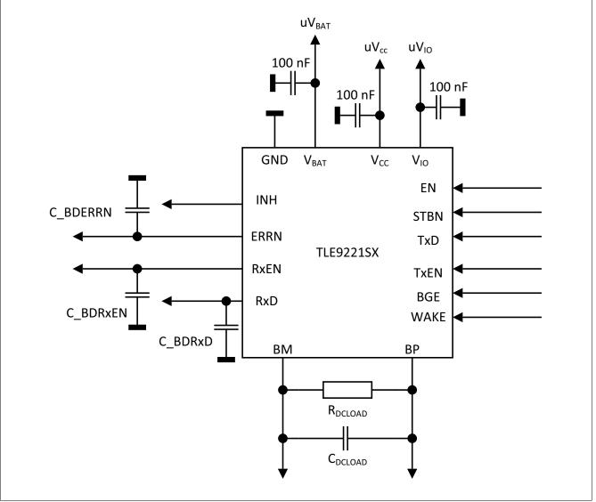
Figure 40 Simplified test circuit
