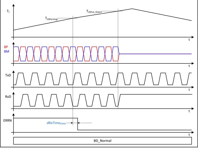
Figure 38 Overtemperature protection
