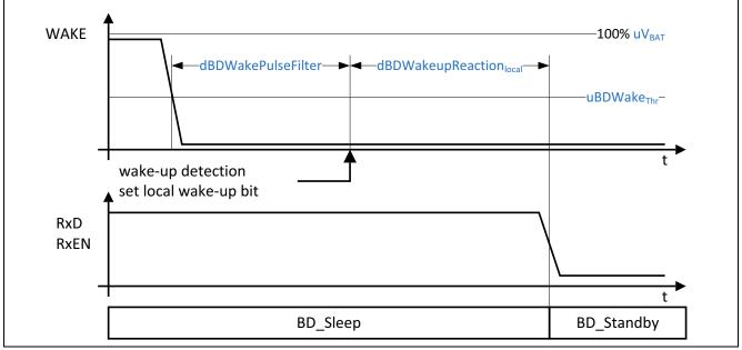
Figure 16 Local wake-up falling edge
