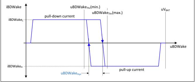
Figure 15 Pull-up and pull-down at the WAKE input
