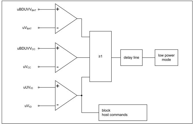
Figure 23 Logic diagram of undervoltage detection
