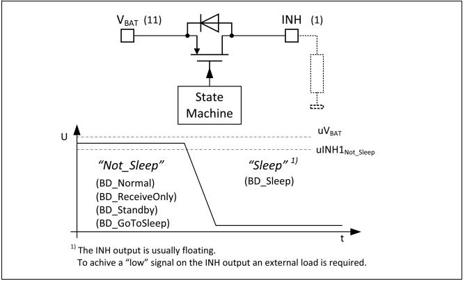
Figure 22 Circuit diagram of the INH output
