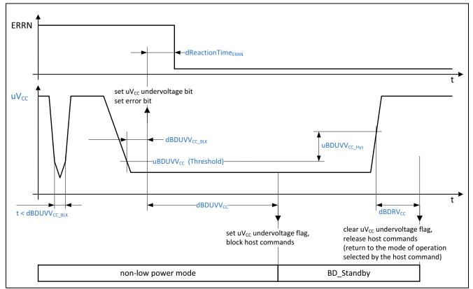
Figure 27 Undervoltage event at uV<sub>cc</sub> in non-low power mode
