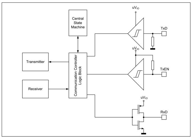
Figure 6 Block diagram of the Communication Controller Interface
