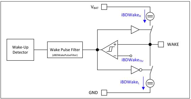
Figure 14 Block diagram of the WAKE input
