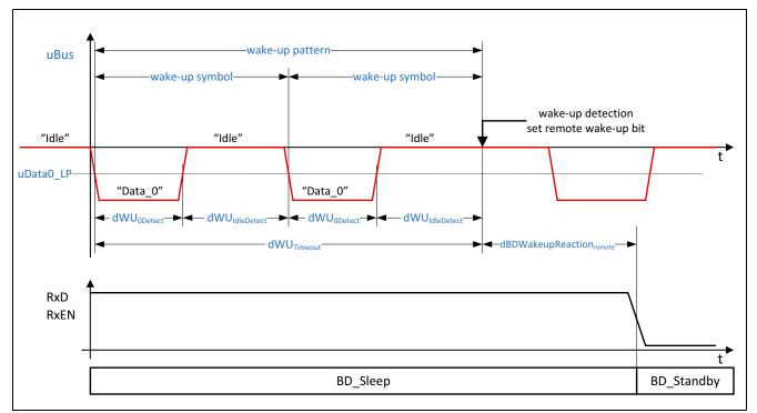
Figure 18 Standard wake-up pattern
