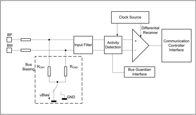
Figure 5 Block diagram of the Receiver
