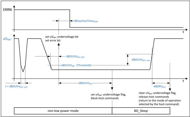
Figure 26 Undervoltage event at uV<sub>BAT</sub> in non-low power mode
