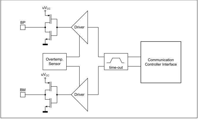
Figure 4 Block diagram of the Transmitter
