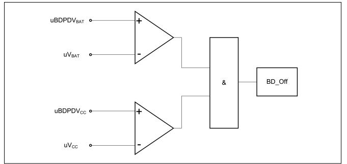
Figure 24 Logic diagram of BD\_Off detection
