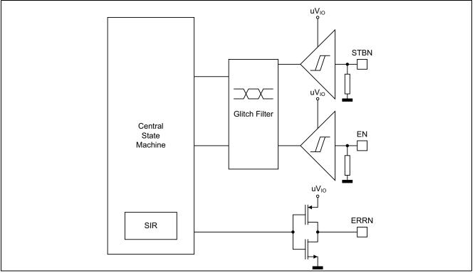
Figure 9 Block diagram of the Host Interface
