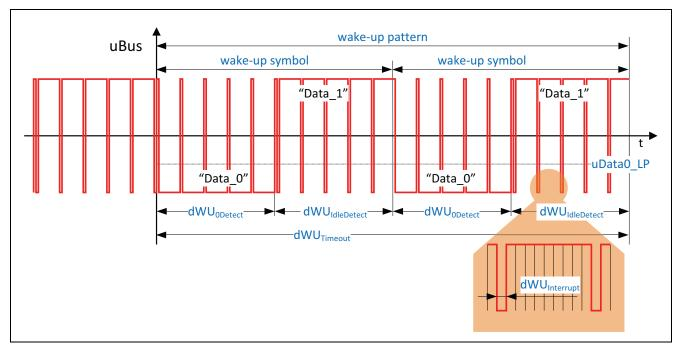
In case any incomplete wake-up pattern is received, no wake-up flag is set and no entry is made to the SIR.
