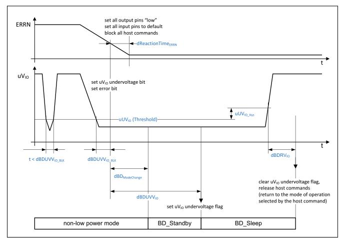
Figure 28 Undervoltage event at uV<sub>10</sub> in non-low power mode
