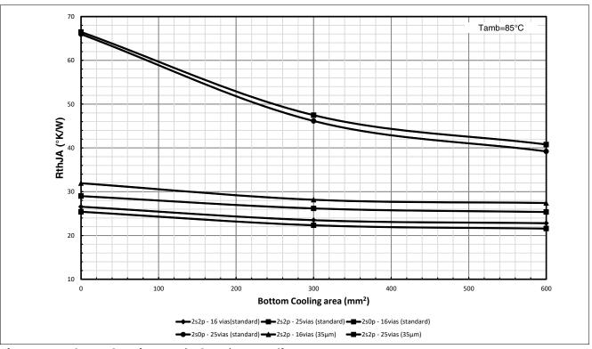
Figure 54 Thermal Resistance (Rth\_JA) vs. Cooling Area
