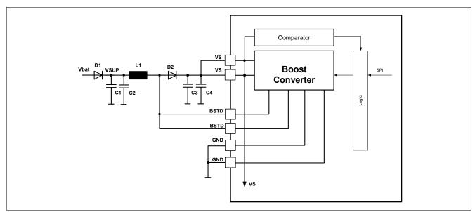
Figure 15 Boost Block Diagram
