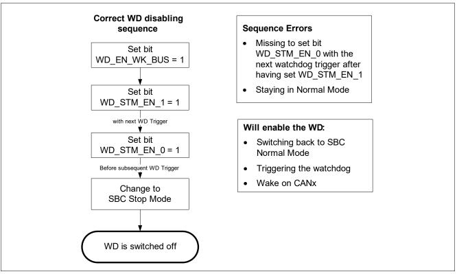
Figure 41 Watchdog Disabling Sequence (with wake via BUS)
