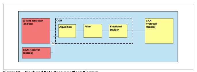
Figure 11 Clock and Data Recovery Block Diagram
