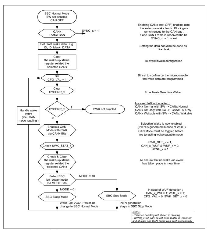
Figure 8 Flow for activation of SWK
