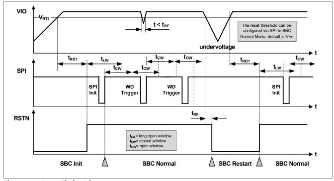
Figure 37 Reset Timing Diagram
