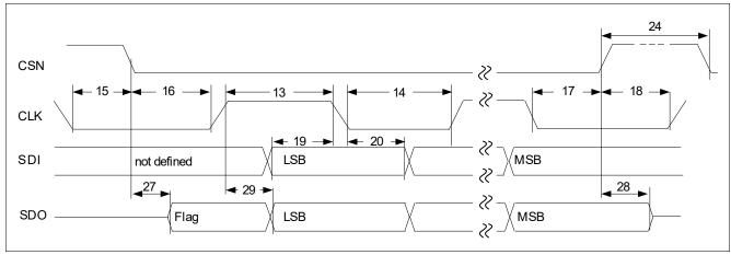
Figure 51 SPI Timing Diagram
