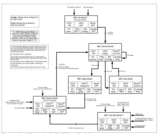
Figure 3 State Diagram showing the SBC Operating Modes
