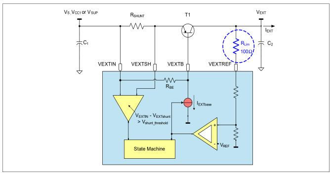
Figure 21 VEXT Hardware Setup
