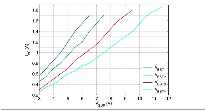
Figure 19 Maximum DCDC Boost current capability versus V<sub>SUP</sub>
