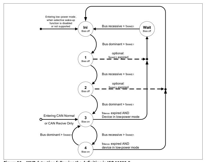
Figure 26 WUP detection following the definition in ISO 11898-5
