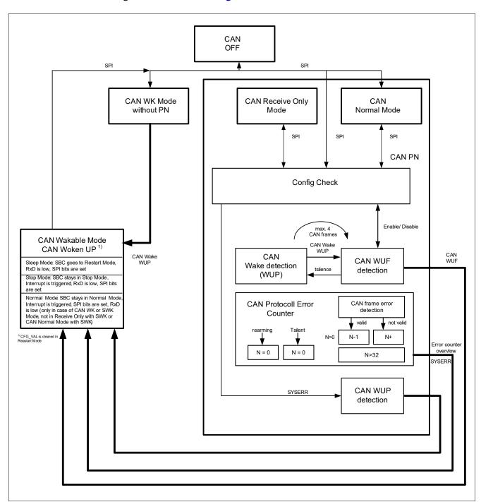
Figure 7 CAN Selective Wake State Diagram
