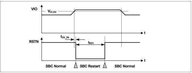
Figure 46 VIO Overvoltage Timing Diagram
