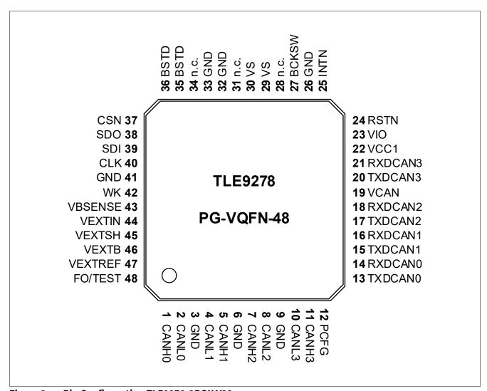
Figure 2 Pin Configuration TLE9278-3BQX V33
