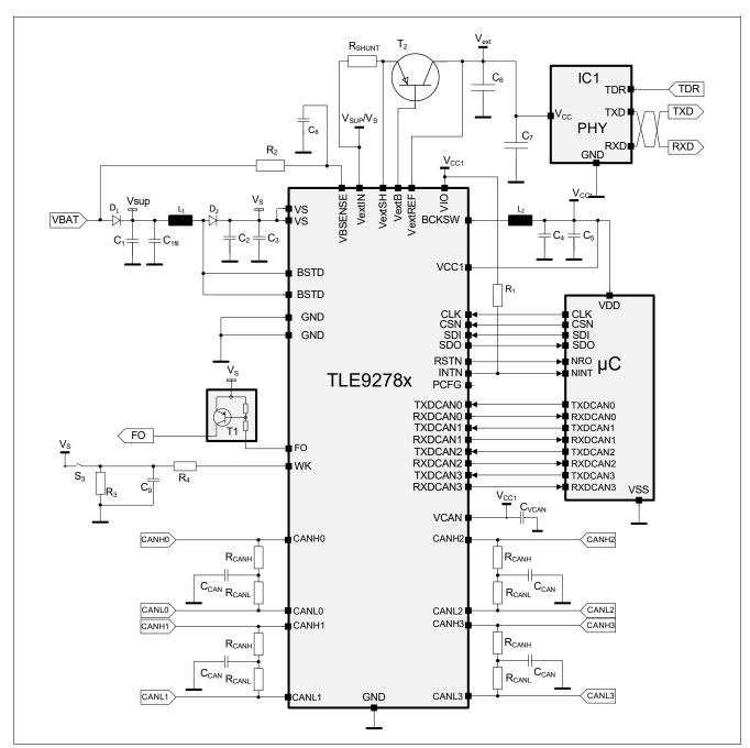
Figure 52 TLE9278-3BQX V33 Application Diagram
