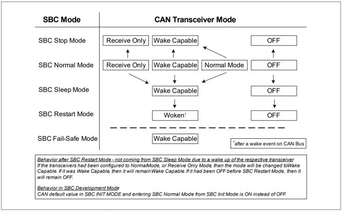
Figure 23 CAN Mode Control Diagram
