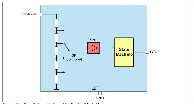
Figure 44 Fast Battery Voltage Monitoring Block Diagram
