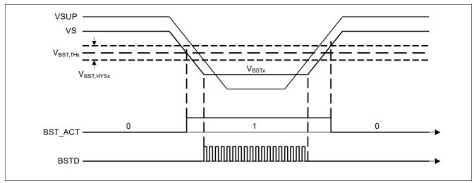
Figure 16 Boost converter activation
