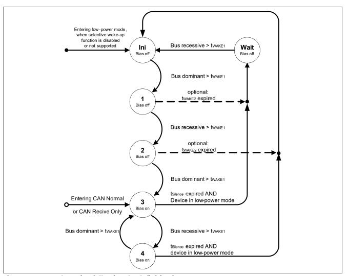
Figure 9 WUP detection following the definition in ISO 11898-5
