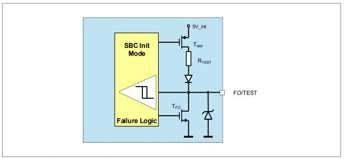
Figure 35 Fail Output Block Diagram
