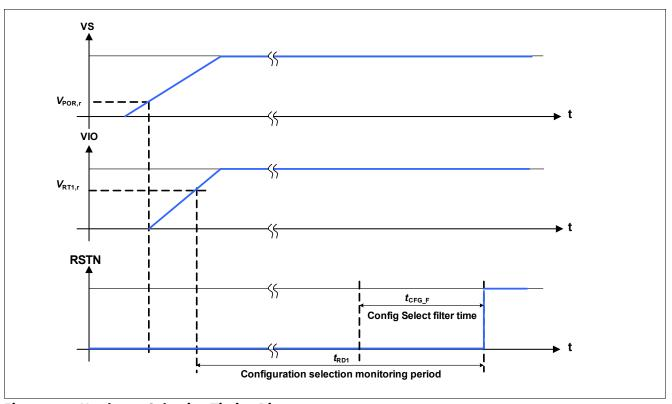
Figure 5 Hardware Selection Timing Diagram
