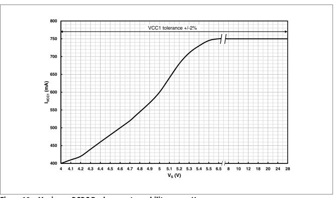
Figure 18 Maximum DCDC Buck current capability versus V<sub>s</sub>
