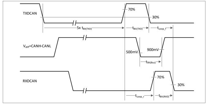
Figure 28 From ISO 11898-2:  $t_{Loop}$ ,  $t_{Bit(TXD)}$ ,  $t_{Bit(RXD)}$  Definition
