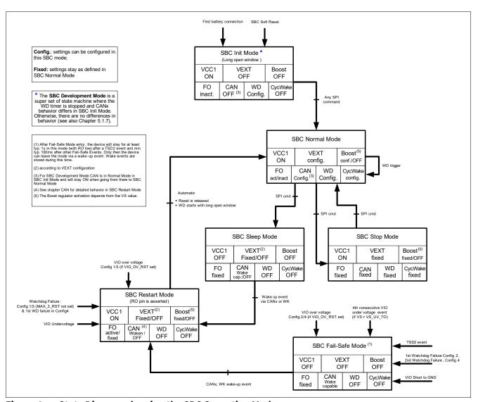
Figure 4 State Diagram showing the SBC Operating Modes
