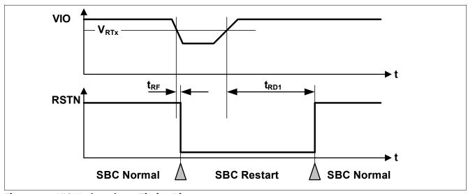
Figure 45 VIO Undervoltage Timing Diagram
