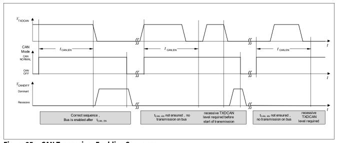
Figure 25 CAN Transceiver Enabling Sequence
