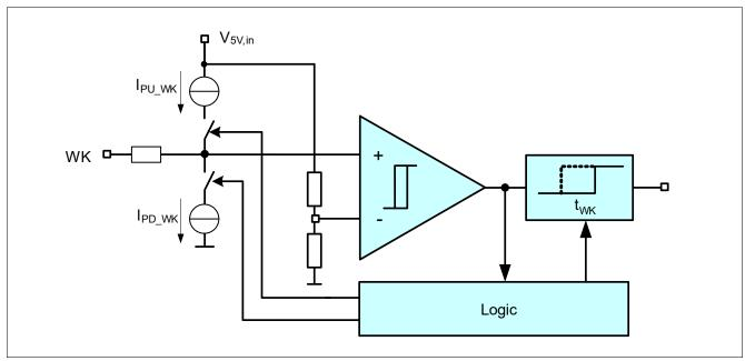
Figure 29 Wake Input Block Diagram
