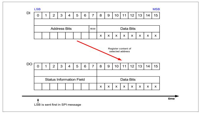
Figure 48 SPI Operation Mode
