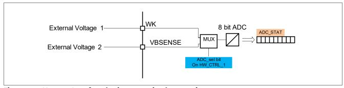
Figure 43 Measure Interface: basic concept implementation.
