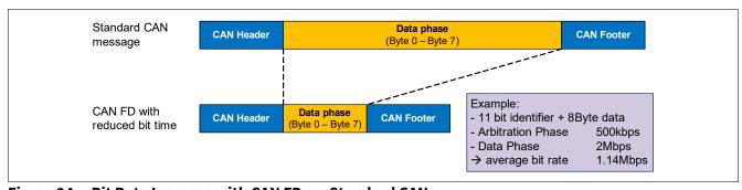
Figure 24 Bit Rate Increase with CAN FD vs. Standard CAN
