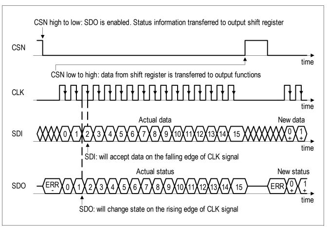
Figure 47 SPI Data Transfer Timing (note the reversed order of LSB and MSB shown in this figure compared to the register description)
