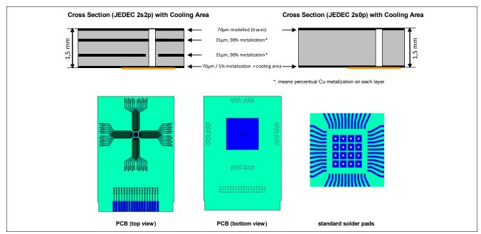
Figure 55 **Board Setup**
