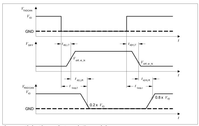
Figure 27 Timing Diagrams for Dynamic Characteristics
