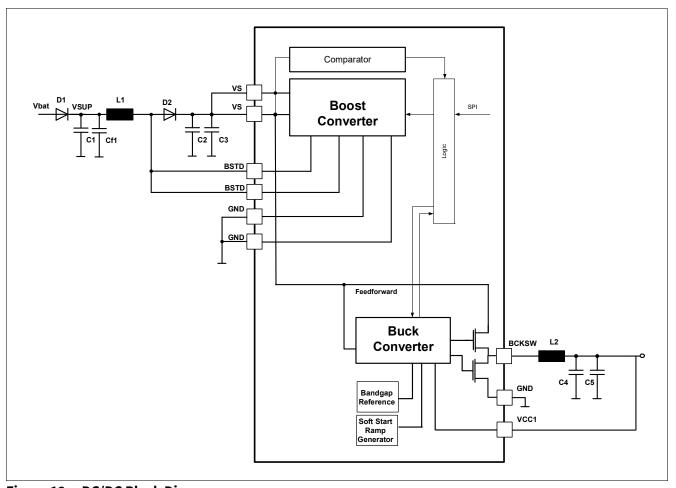
Figure 12 DC/DC Block Diagram
