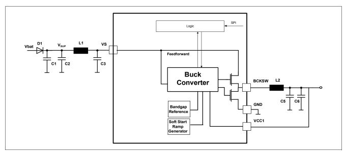
Figure 13 Buck Block Diagram
