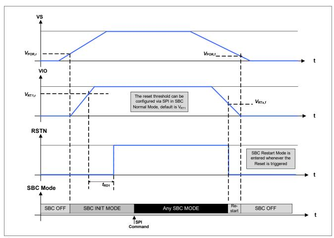
Figure 42 Ramp up / down example of Supply Voltage
