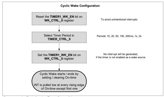
Figure 6 **Cyclic Wake: Configuration and Sequence**
