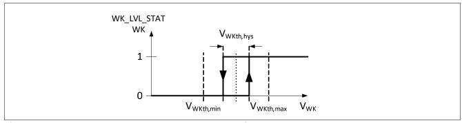
Figure 30 Wake Input Threshold Levels and Hysteresis
