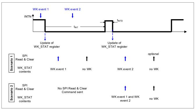
Figure 34 Interrupt Signaling Behavior
